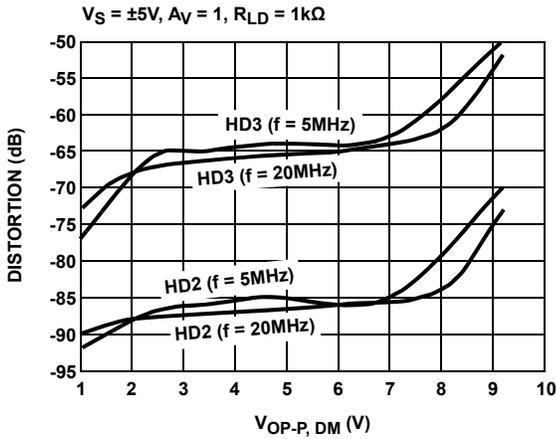
FIGURE 13. HARMONIC DISTORTION vs DIFFERENTIAL OUTPUT VOLTAGE
