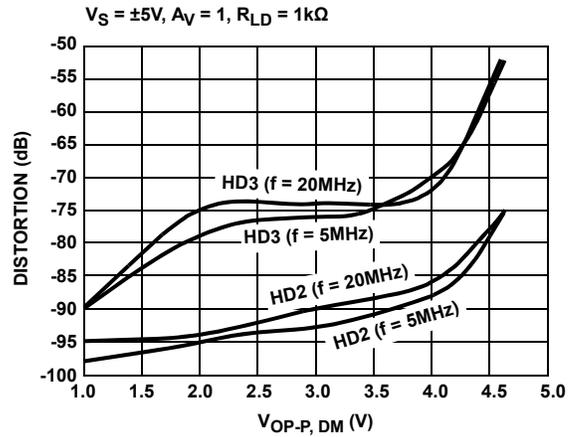
FIGURE 12. HARMONIC DISTORTION vs DIFFERENTIAL OUTPUT VOLTAGE
