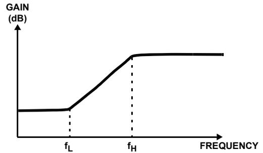
$$\text{DC Gain} = 1 + \frac{2R_F}{R_G}$$
