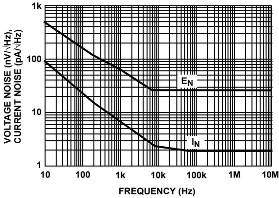
FIGURE 11. VOLTAGE AND CURRENT NOISE vs FREQUENCY
