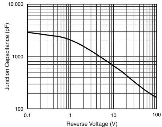
Fig. 5 - Typical Junction Capacitance Per Diode
