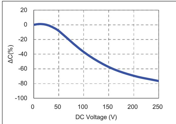
4) Bias TCC characteristics (Agilent 4284A, 1kHz, 1Vrms, 125Vdc)
