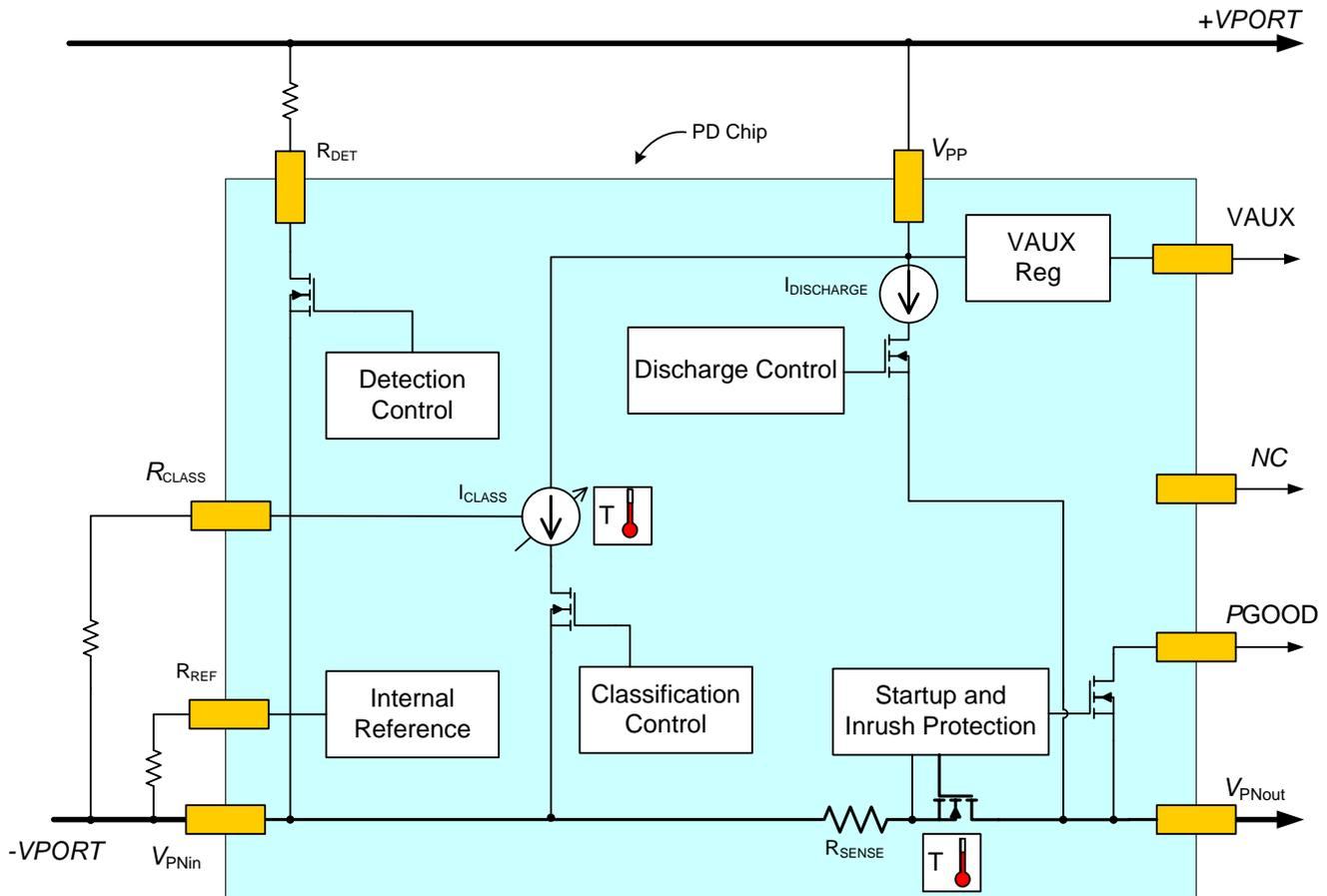
Figure 1: PD70100 Functional Block Diagram
