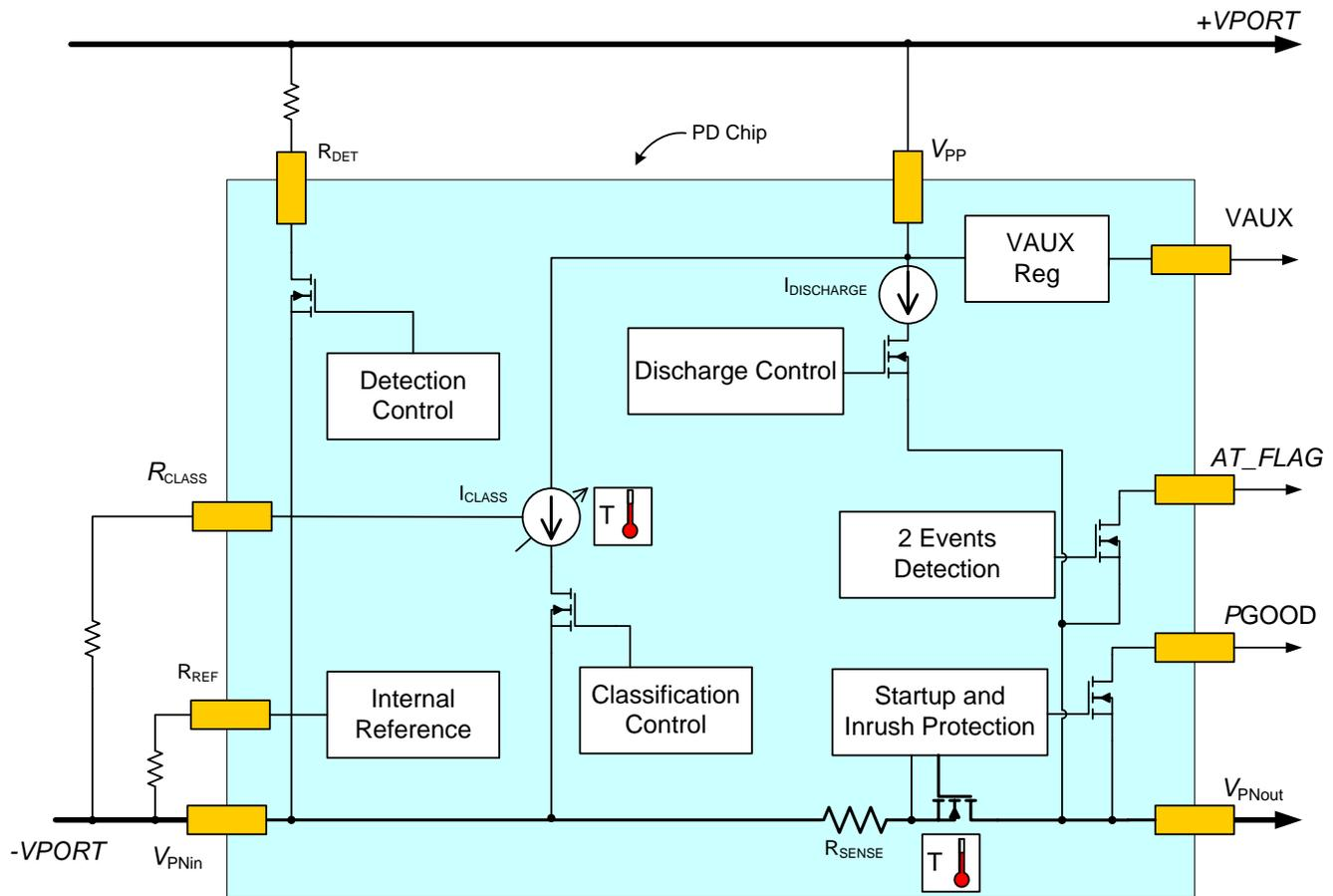
Figure 2: PD70200 Functional Block Diagram
