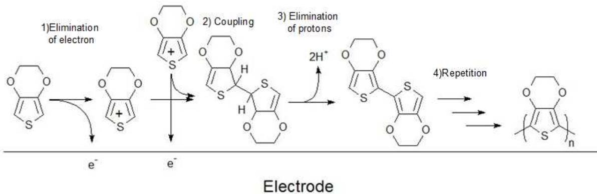
Fig-1 PEDOT Polymerization process
