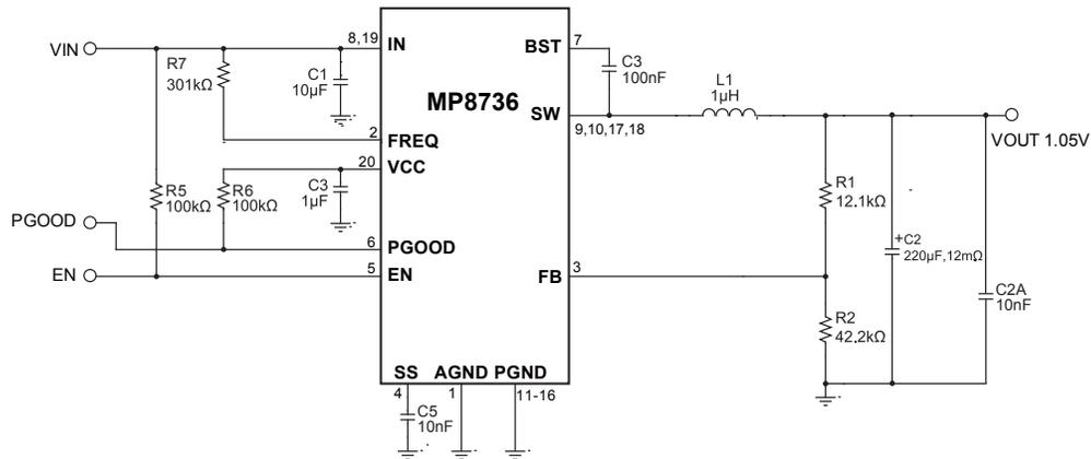
**Figure 12—Typical Application Circuit with No External Ramp**
