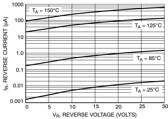
Figure 3. Leakage Current
