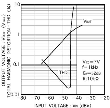
Fig.11 Input/output characteristics
