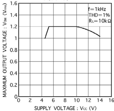
Fig.12 Maximum output voltage vs. power supply voltage
