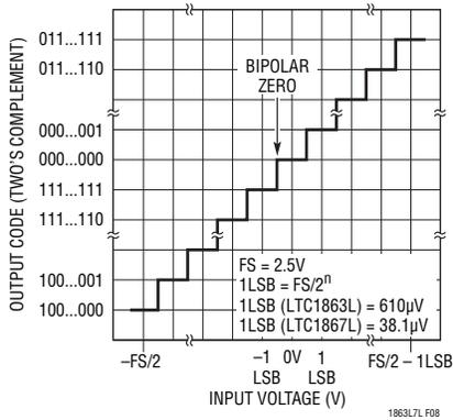
**Figure 8. LTC1863L/LTC1867L Bipolar Transfer Characteristics (Two's Complement)**
