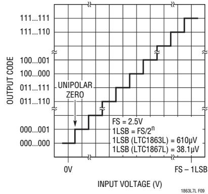
**Figure 9. LTC1863L/LTC1867L Unipolar Transfer Characteristics (Straight Binary)**
