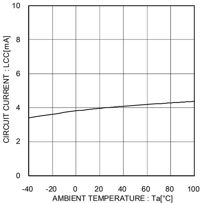
Figure 6. Circuit Current
