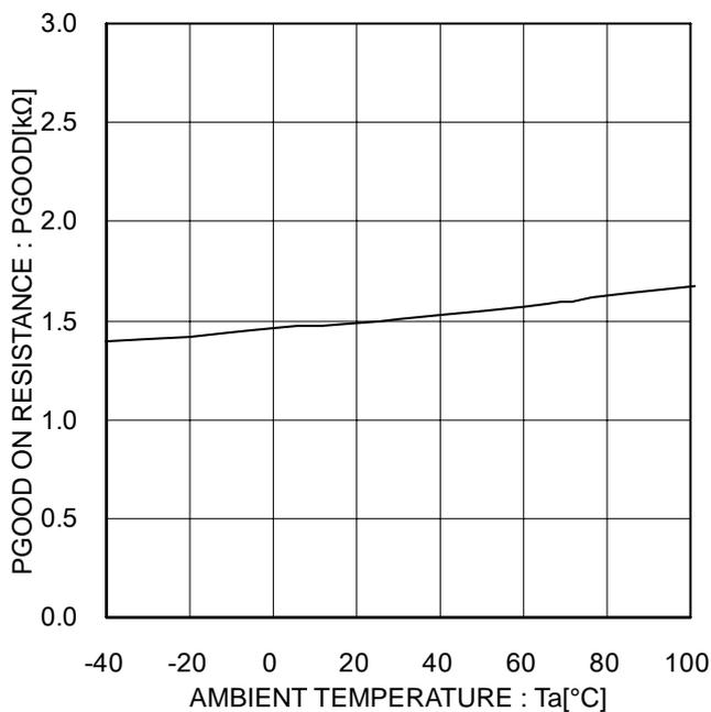
Figure 14. PGOOD Pin ON Resistance vs. Temperature Characteristics
