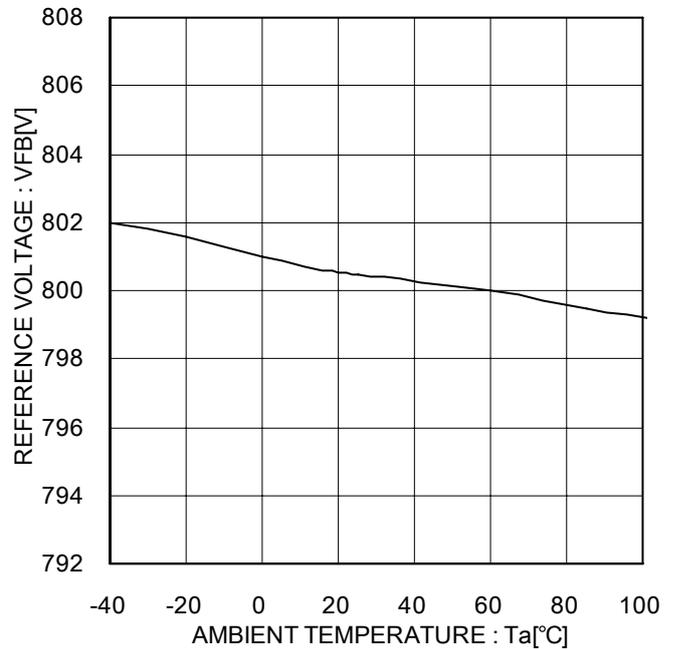
Figure 7. Reference Voltage vs. Temperature Characteristics
