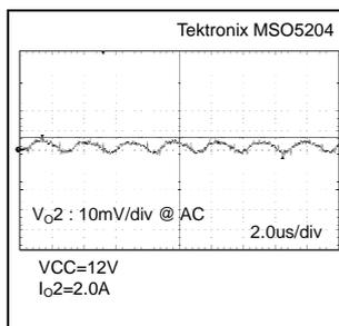
Figure 38. Output Ripple voltage ( $V_{O2}=3.3V$ )
