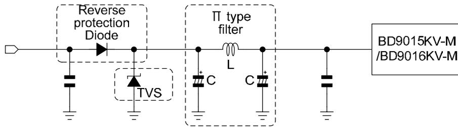
Figure 41. Filter circuit
