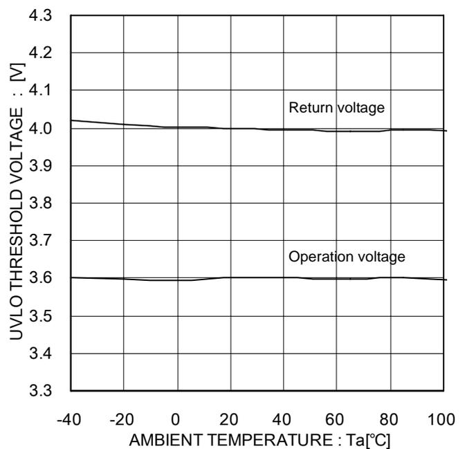
Figure 11. UVLO Operation/Return Voltage vs. Temperature Characteristics
