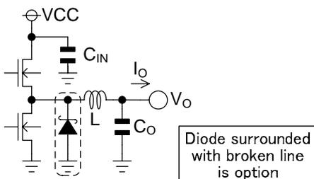
Figure 20. Input Capacitor
