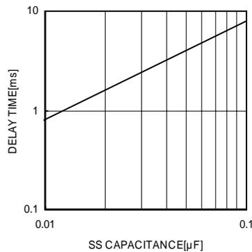
$$T_{SS} = \frac{0.8V(Typ) \times C_{SS}}{I_{SS} (10\mu A (Typ))} \text{ [sec]}$$
