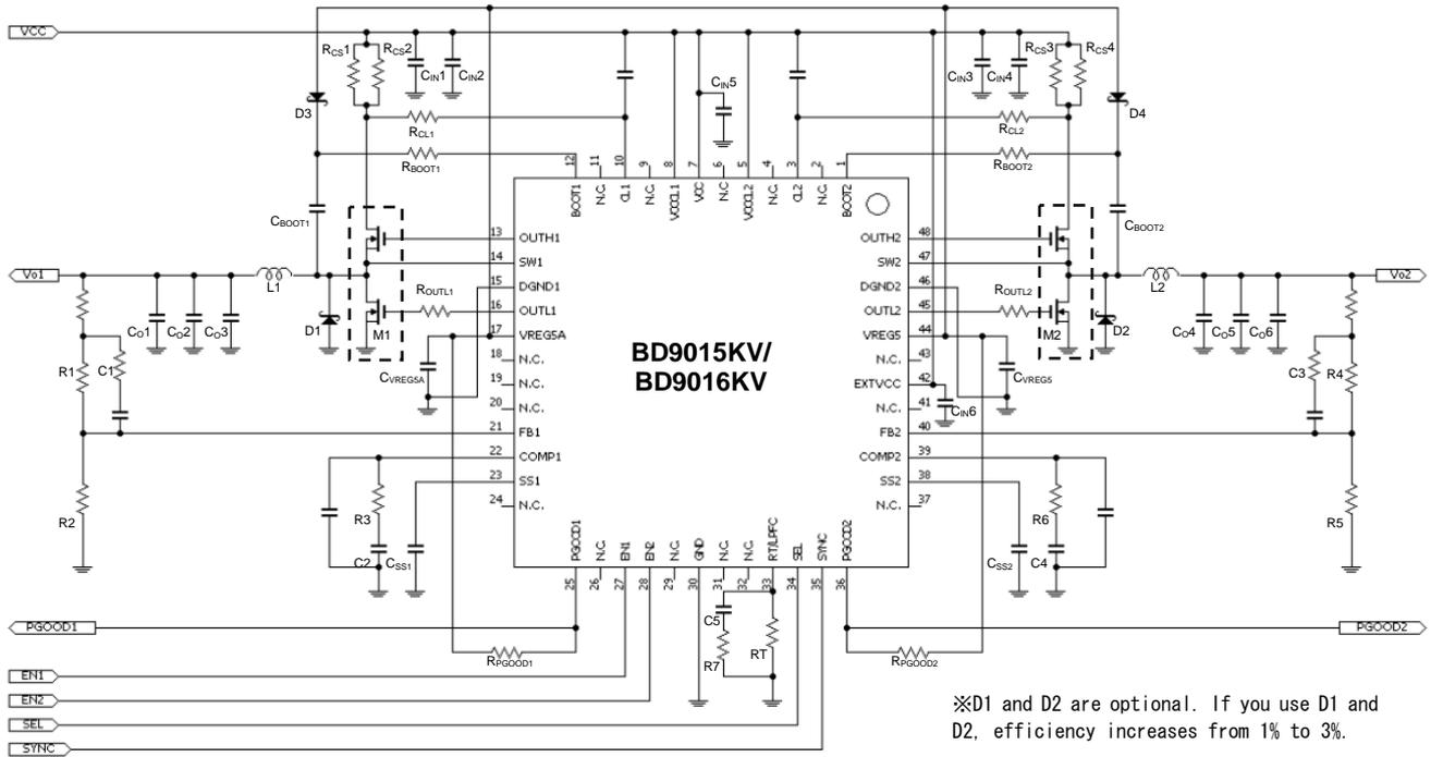
Figure 32. Reference circuit
