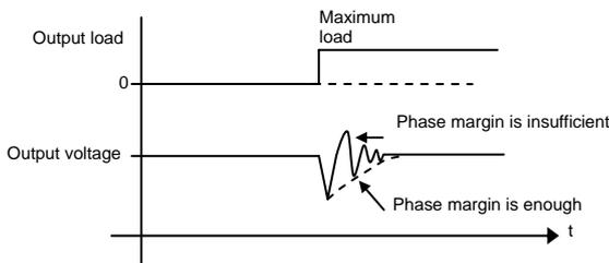
The phase margin can also be measured with the load responsiveness. Measure the variation in output voltage when instantaneously changing the load from no load to maximum load. If ringing occurs, the phase margin is insufficient. If no ringing occurs, the phase margin is sufficient. The actual phase margin can not be measured.
