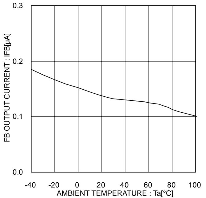
Figure 13. FB Pin Source Current vs. Temperature Characteristics
