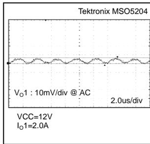
Figure 34. Output Ripple voltage ( $V_{O1}=5V$ )
