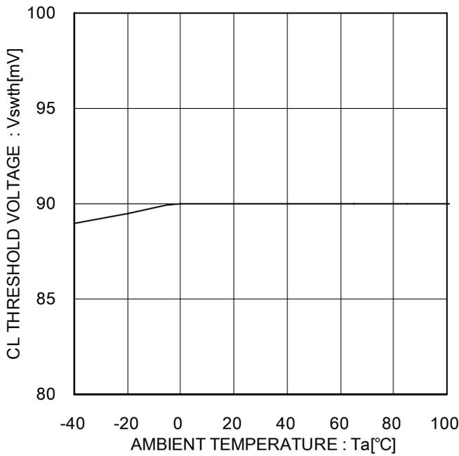
Figure 8. CL Pin Threshold Voltage vs. Temperature Characteristics
