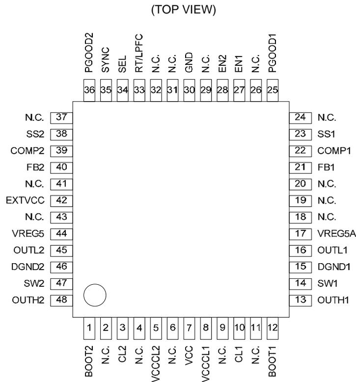
Figure 2. Pin Configuration
