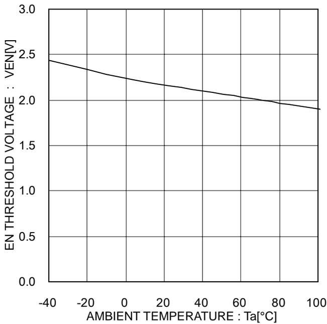
Figure 12. EN Threshold Voltage vs. Temperature Characteristics
