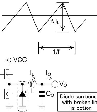
Figure 19. Output Ripple Current
