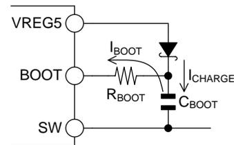
Figure 29. Setting the BOOT pin Serial Resistors
