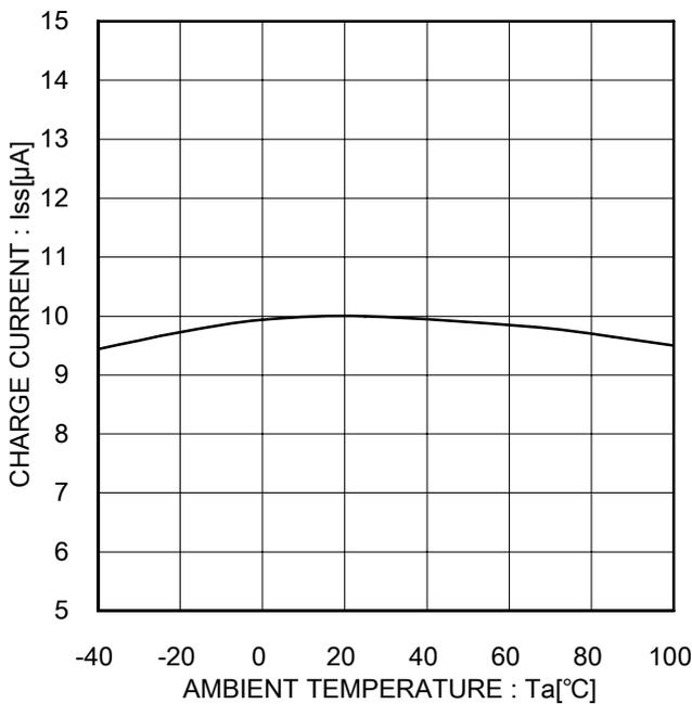
Figure 10. SS Charge Current vs. Temperature Characteristics
