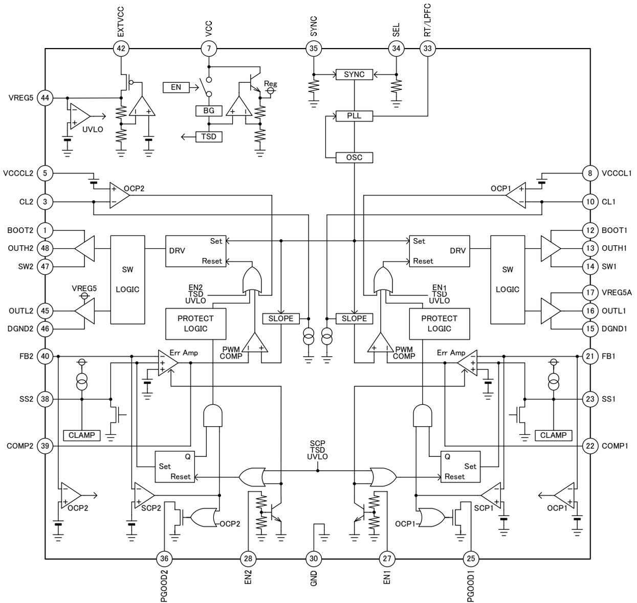
Figure 3. Block Diagram
