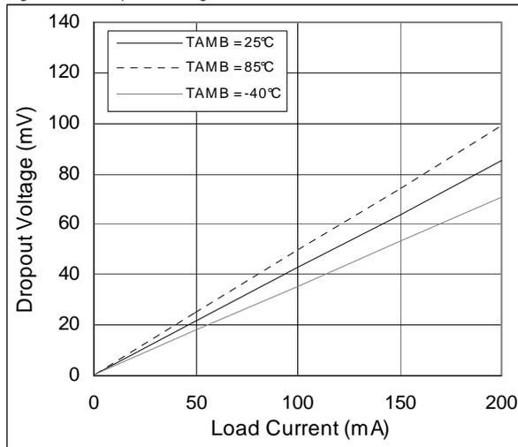
Figure 11.  $V_{OUT}$  vs.  $I_{OUT}$ ;  $V_{OUT(NOM)}=1.5V$
