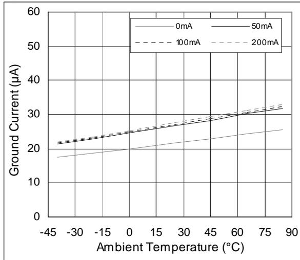
Figure 24. Ground Current vs. Temperature;  $V_{OUT}=2.8V$
