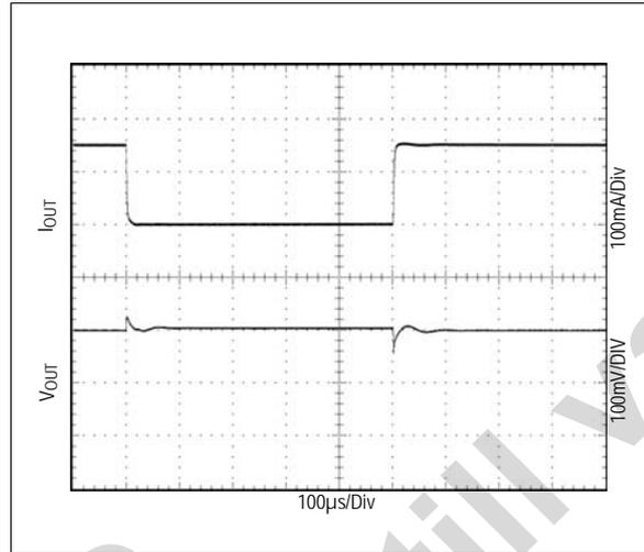
Figure 42. Load Transient;  $I_{OUT}=0mA$  to  $150mA$
