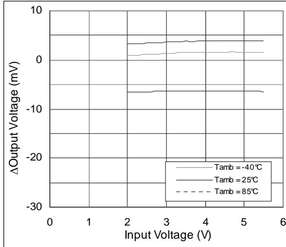
Figure 6.  $\Delta V_{OUT}$  vs.  $V_{IN}$ ;  $V_{OUT(NOM)}=2.8V$
