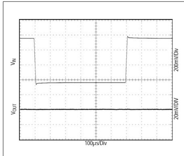
Figure 40. Load Transient;  $I_{OUT}=0mA$  to  $150mA$
