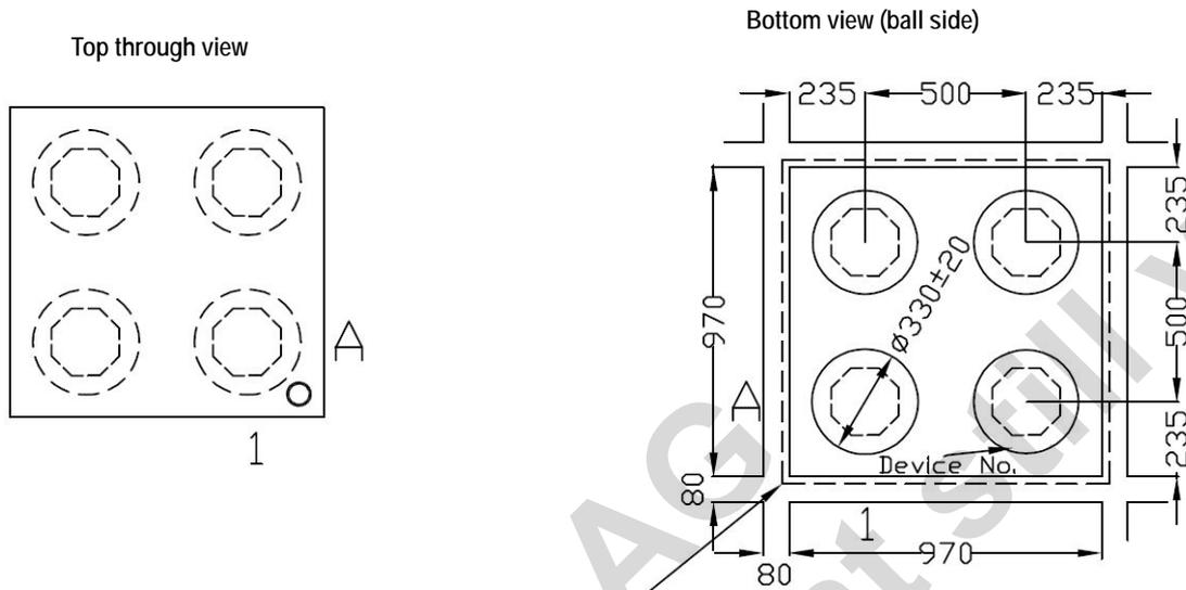
Die size after cutting 1015x1015 ±20µm
