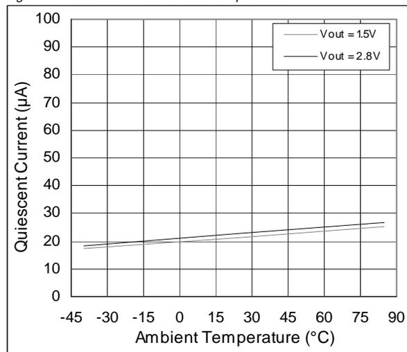
Figure 23. Ground Current vs. Temperature;  $V_{OUT}=1.5V$
