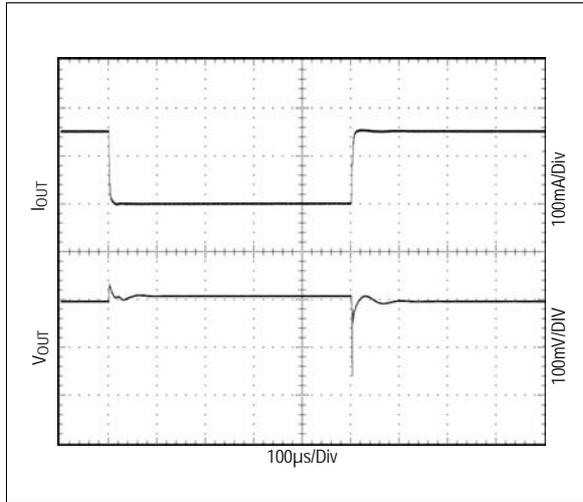
Figure 41. Load Transient;  $I_{OUT}=0mA$  to  $150mA$
