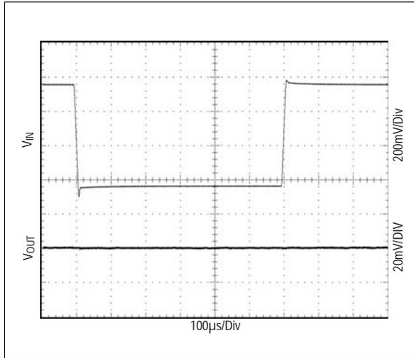
Figure 35. Line Transient Response;  $I_{OUT}=50\text{mA}$ ,  $V_{OUT}=2.8\text{V}$ ,
