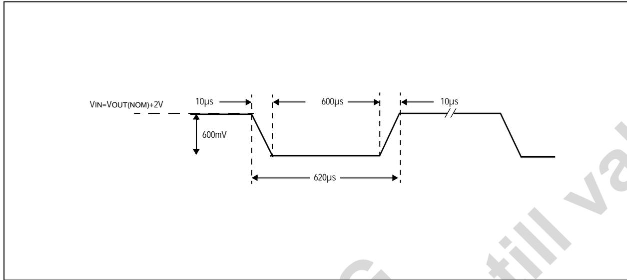
Figure 4. SVR Input Voltage Test Signal
