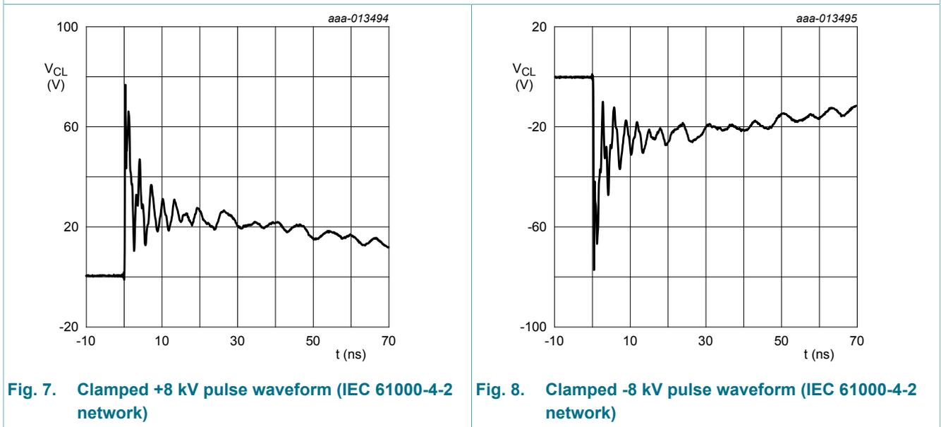
Fig. 7. Clamped +8 kV pulse waveform (IEC 61000-4-2 network)
