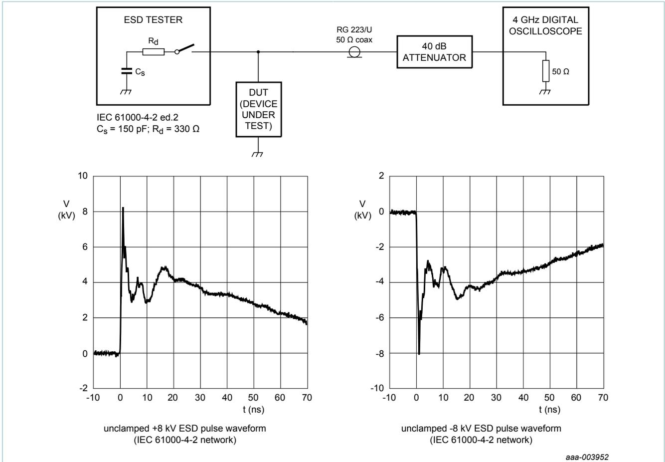
Fig. 6. ESD clamping test setup and waveforms
