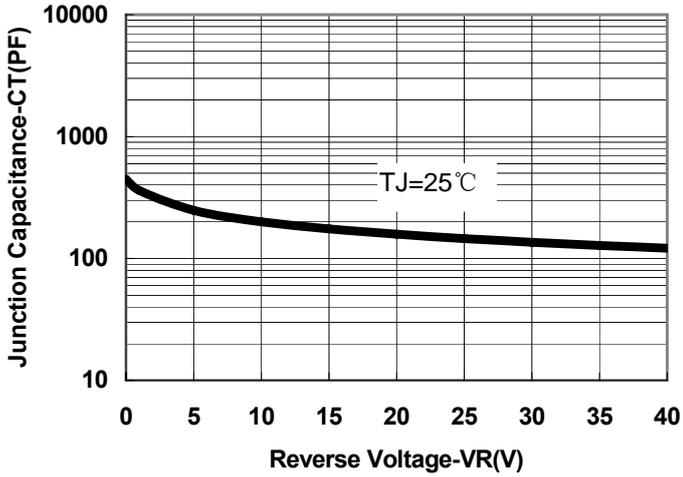
Fig.1-Typical Junction Capacitance
