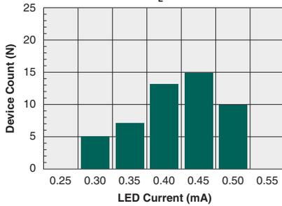
Typical I<sub>F</sub> for Switch Dropout
