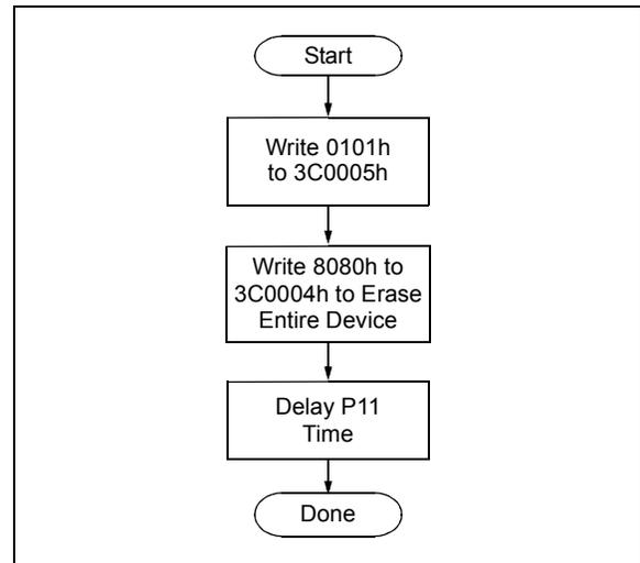
**FIGURE 3-2: BULK ERASE TIMING**
