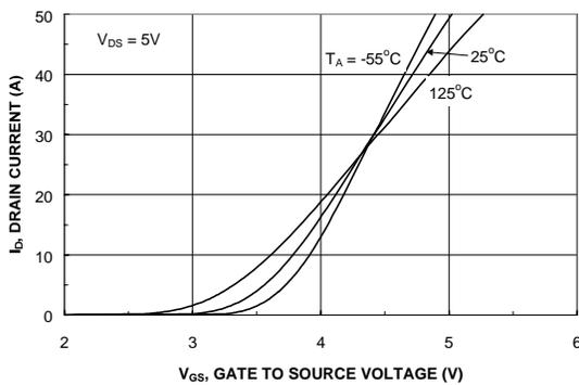
Figure 5. Transfer Characteristics.
