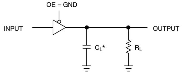
\*Includes all probe and jig capacitance.
