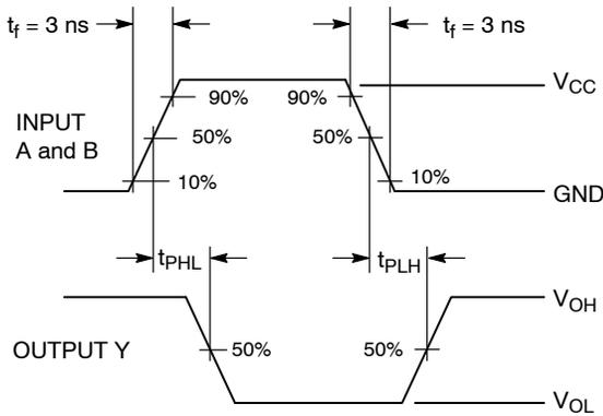
**Figure 3. Switching Waveform**
