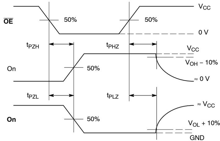
**Figure 5. AC Output Enable and Disable Waveform**
