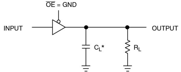
\*Includes all probe and jig capacitance.
