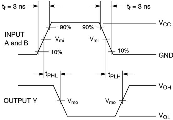
**Figure 3. Switching Waveform**
