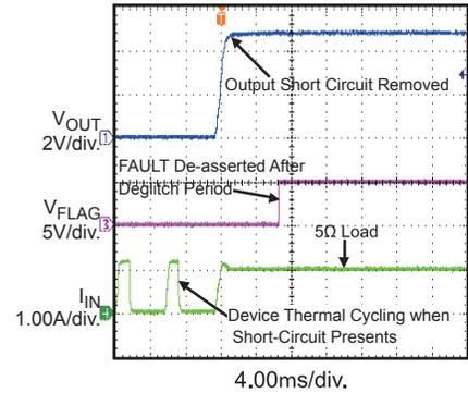
**No-Load to Short-Circuit Transient Response**
