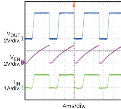
**Figure 7—Auto-Retry Waveform**
