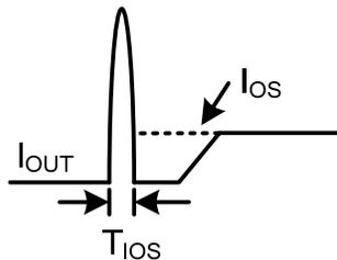
**Figure 2—Short Circuit Response Time**
