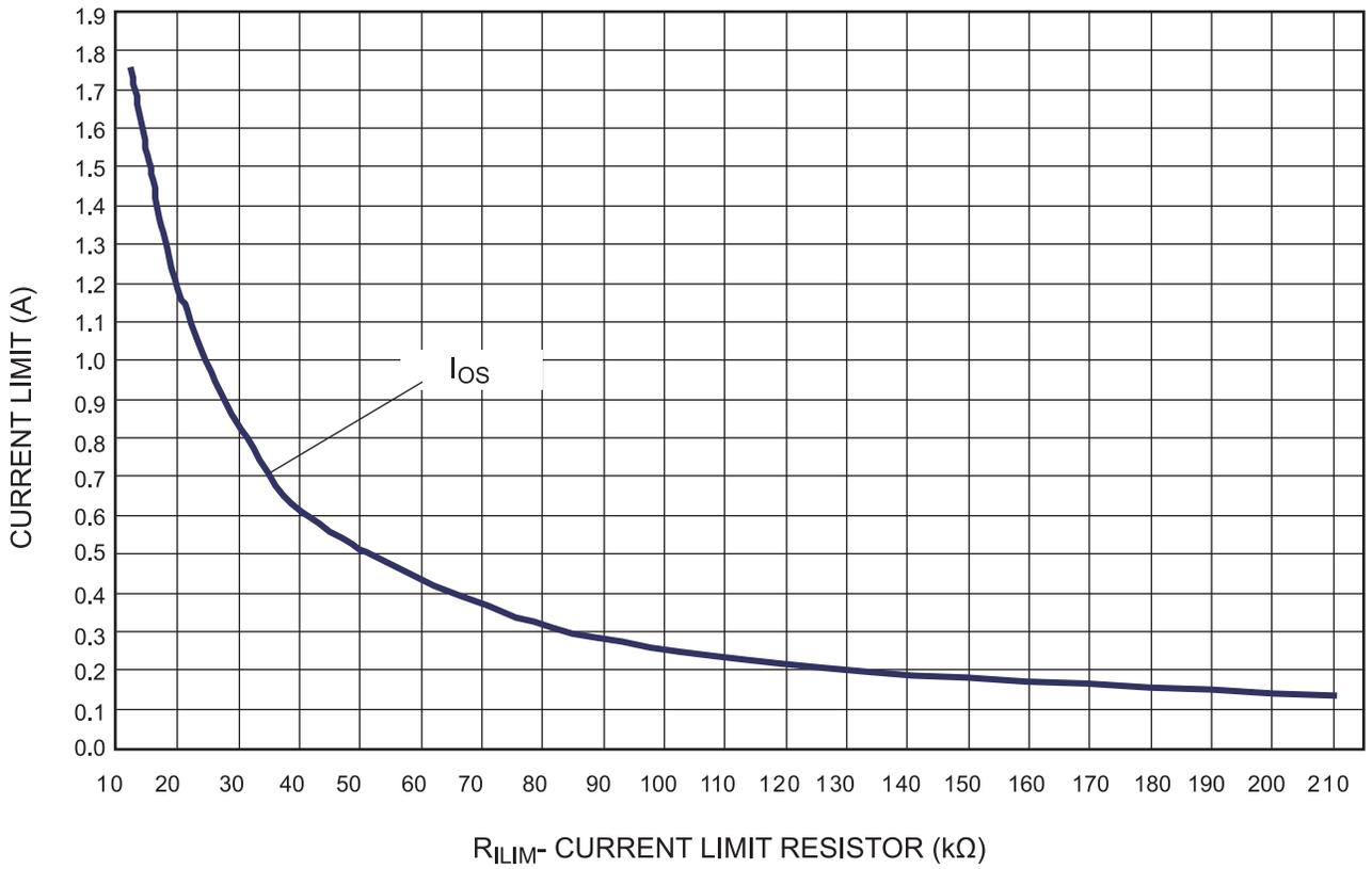
**Figure 5—Current-Limit vs R<sub>ILIM</sub>**
