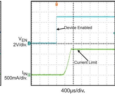
**1Ω Load Connected to Enabled Device**
