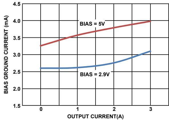
FIGURE 13. BIAS GROUND CURRENT vs LOAD CURRENT
