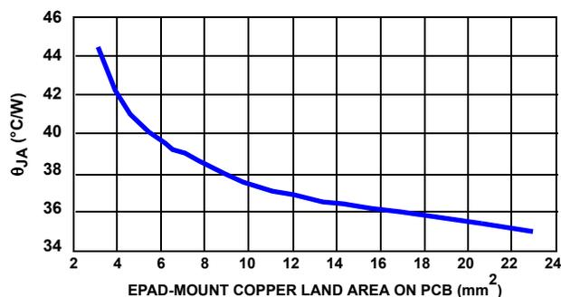
FIGURE 38. 3mmx3mm-10 PIN DFN ON 4-LAYER PCB WITH THERMAL VIAS θ<sub>JA</sub> vs EPAD-MOUNT COPPER LAND AREA ON PCB
