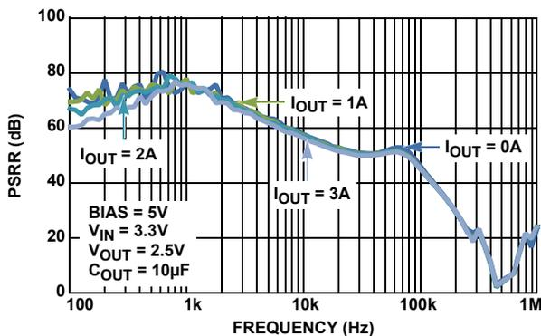
FIGURE 3.  $V_{IN}$  PSRR vs LOAD CURRENT (ISL80113)
