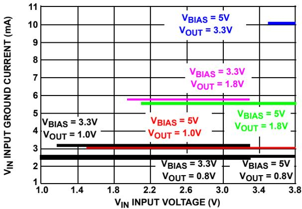
FIGURE 14. INPUT GROUND CURRENT vs  $V_{\text{IN}}$  and  $V_{\text{OUT}}$
