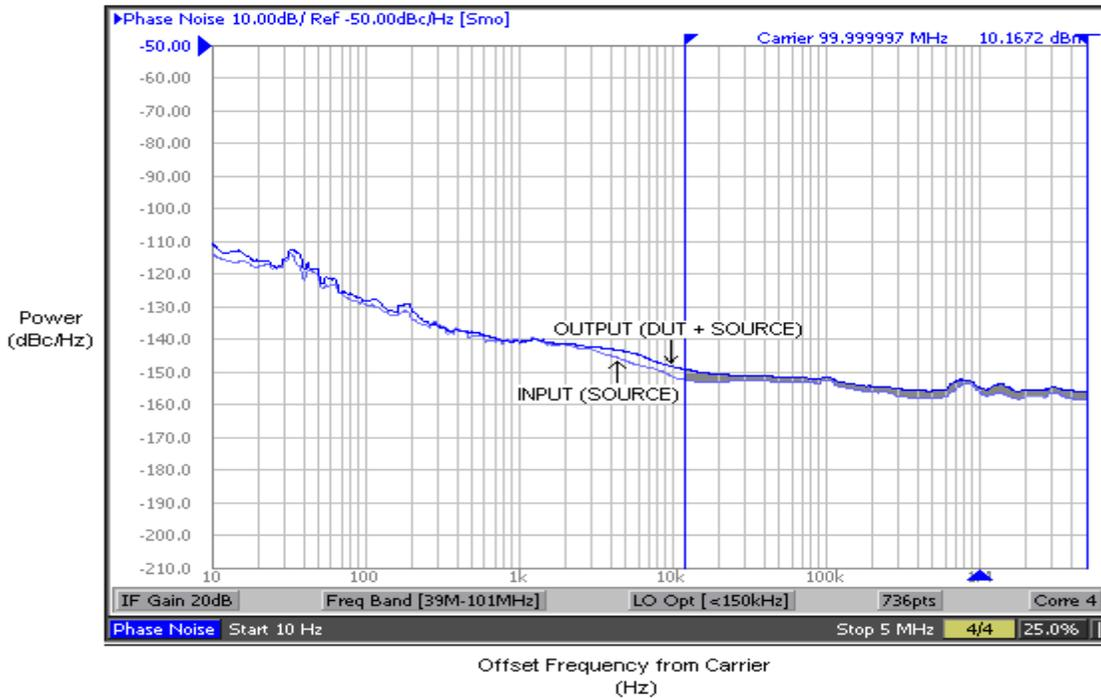
The above plot captured using Agilent E5052A shows Additive Phase Noise of the NB3L553 device measured with an input source generated by Agilent E8663B. The RMS phase jitter contributed by the device (integrated between 12 kHz to 20 MHz; as shown in the shaded area) is 18 fs (RMS Phase Jitter of the input source is 75.40 fs and Output (DUT+Source) is 93.16 fs).
