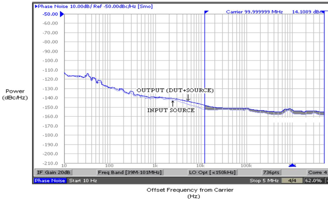
The above plot captured using Agilent E5052A shows Additive Phase Noise of the NB3L553 device measured with an input source generated by Agilent E8663B. The RMS phase jitter contributed by the device (integrated between 12 kHz to 20 MHz; as shown in the shaded area) is 29 fs (RMS Phase Jitter of the input source is 75.40 fs and Output (DUT+Source) is 103.85 fs).
