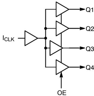
Figure 1. Block Diagram
