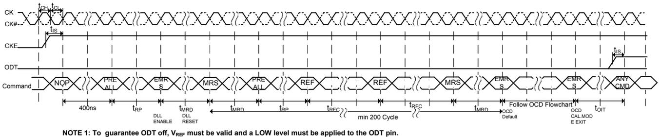
**Figure 8. ODT update delay timing- $t_{MOD}$**
