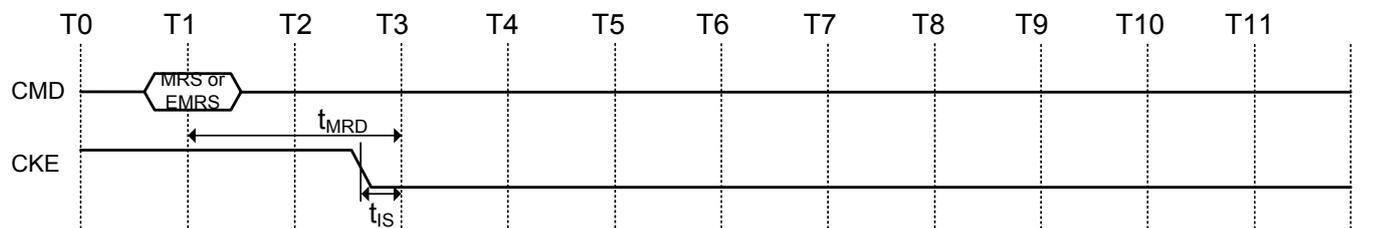
**Figure 56. Asynchronous CKE LOW event**
