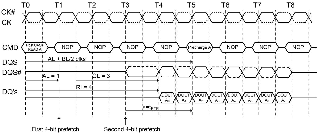
**Figure 32. Burst read operation followed by precharge:**
