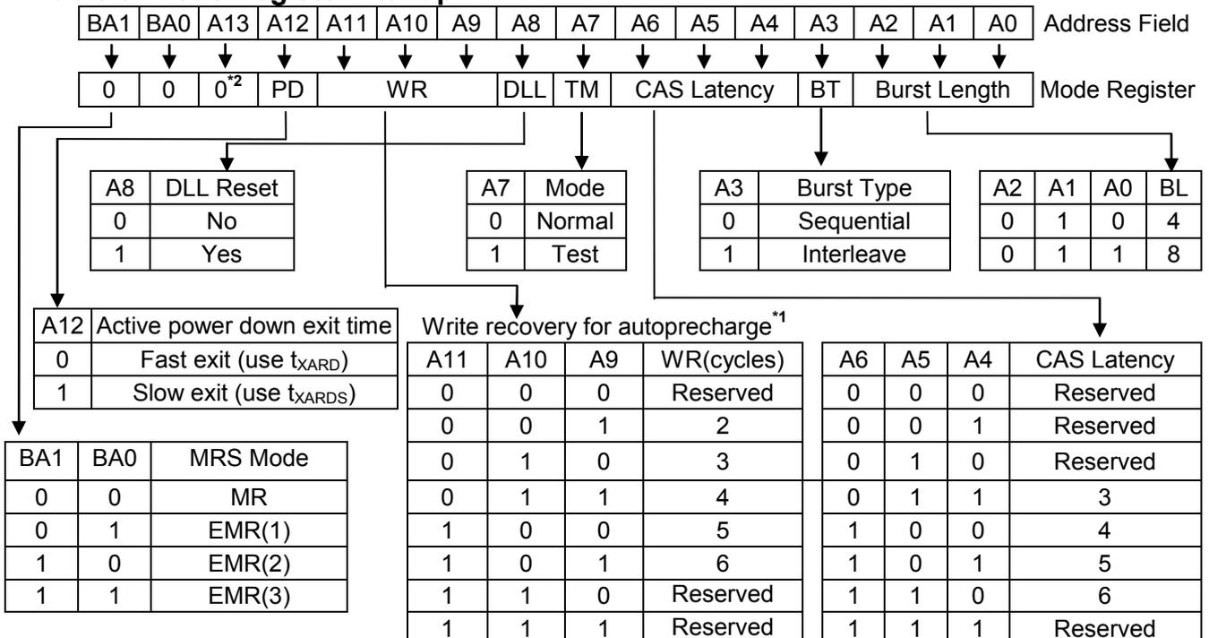
**NOTE 1:** For DDR2-667/800, WR min is determined by  $t_{CK}(\text{avg})$  max and WR max is determined by  $t_{CK}(\text{avg})$  min.  $WR[\text{cycles}] = RU \{t_{WR}[\text{ns}]/t_{CK}(\text{avg})[\text{ns}]\}$ , where RU stands for round up. The mode register must be programmed to this value. This is also used with  $t_{RP}$  to determine  $t_{DAL}$ .
