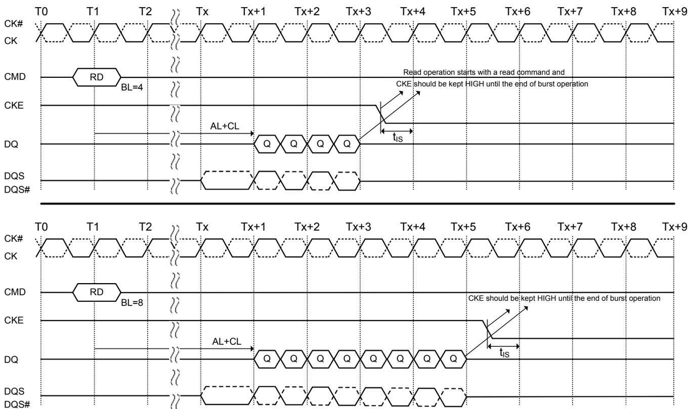
**Figure 49. Read with autoprecharge to power-down entry**
