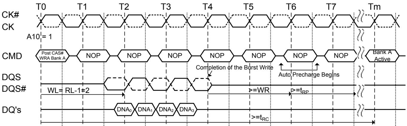
**Figure 42. Burst write with auto-precharge (WR+t<sub>RP</sub>): WL=4, WR=2, BL=4, t<sub>RP</sub>=3**
