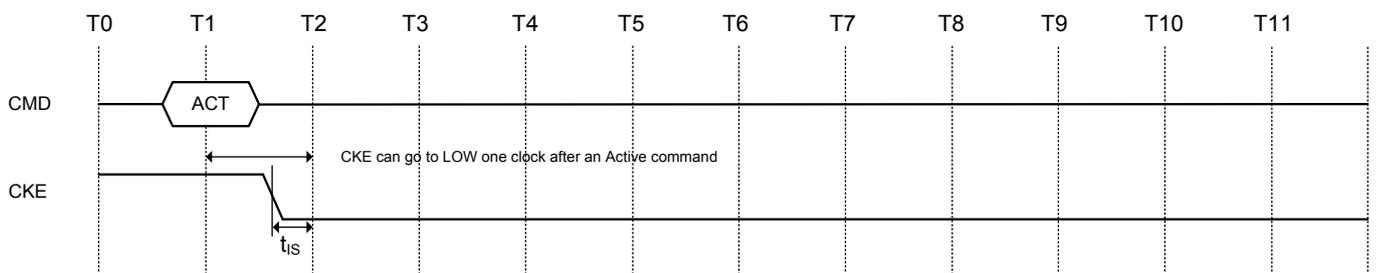
**Figure 54. Precharge/precharge-all command to power-down entry**
