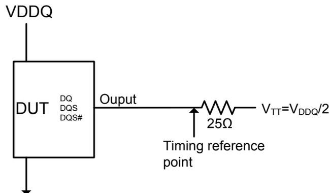
The output timing reference voltage level for single ended signals is the crosspoint with  $V_{TT}$ . The output timing reference voltage level for differential signals is the crosspoint of the true (e.g. DQS) and the complement (e.g. DQS#) signal.
