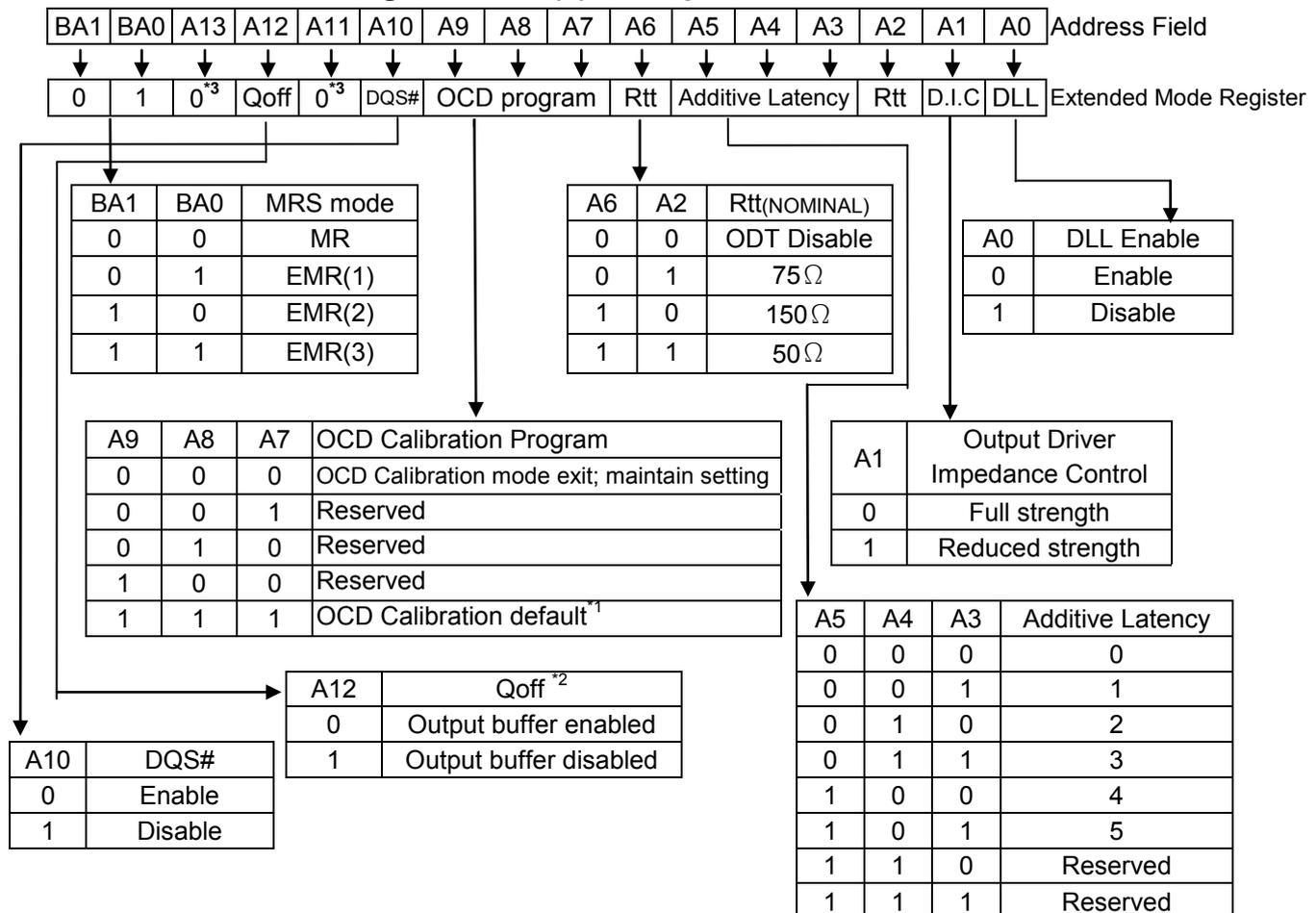
**NOTE 1:** After setting to default, OCD calibration mode needs to be exited by setting A9-A7 to 000.
