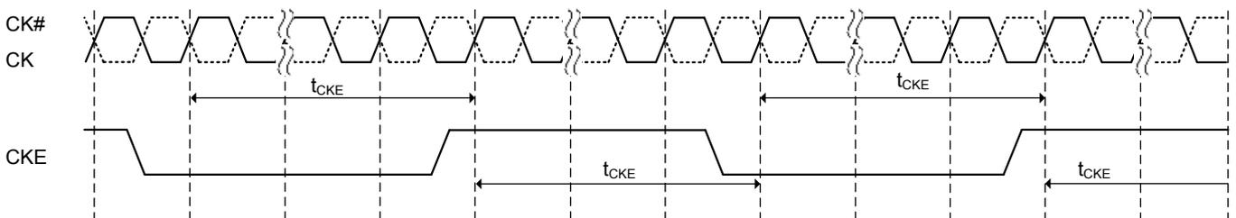
NOTE: DRAM guarantees all AC and DC timing & voltage specifications and proper DLL operation with intensive CKE operation
