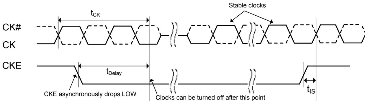
**Figure 57. Clock frequency change in precharge power down mode**
