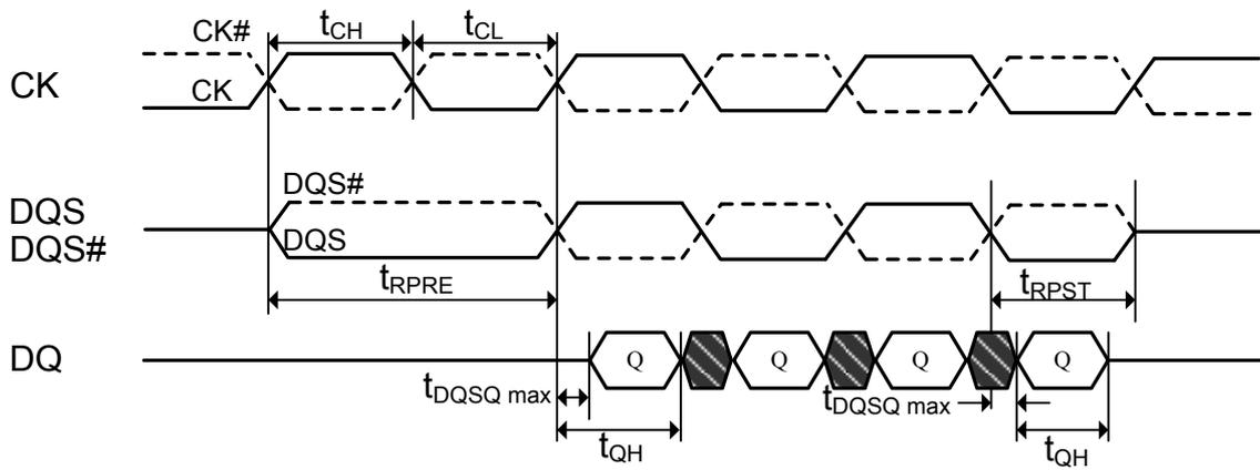
**Figure 18. Data input (write) timing**
