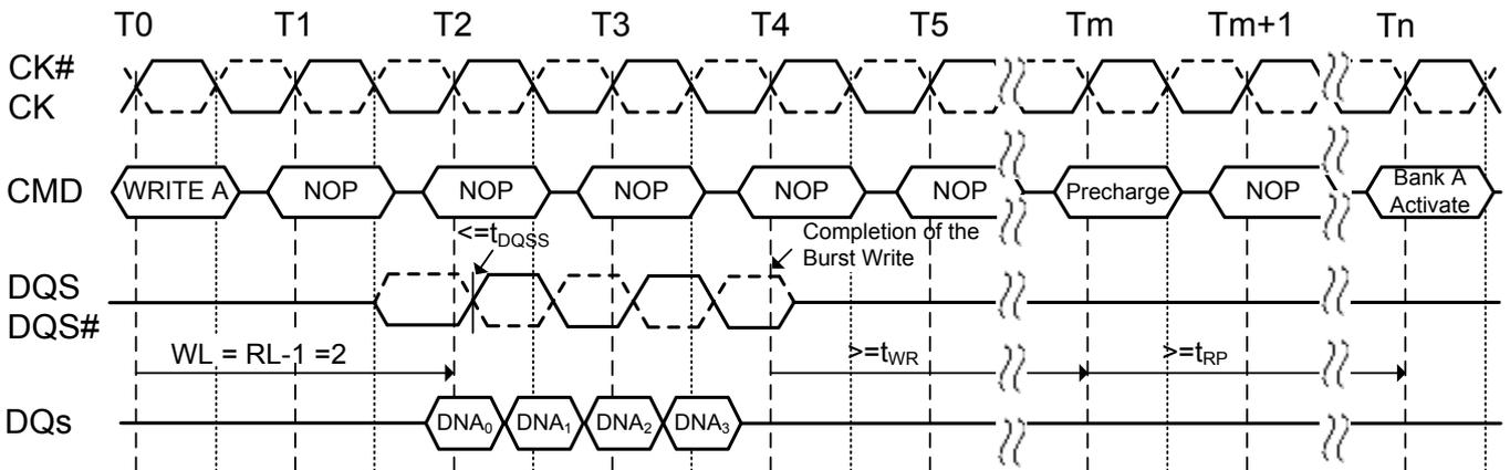
**Figure 26. Burst write followed by burst read:
