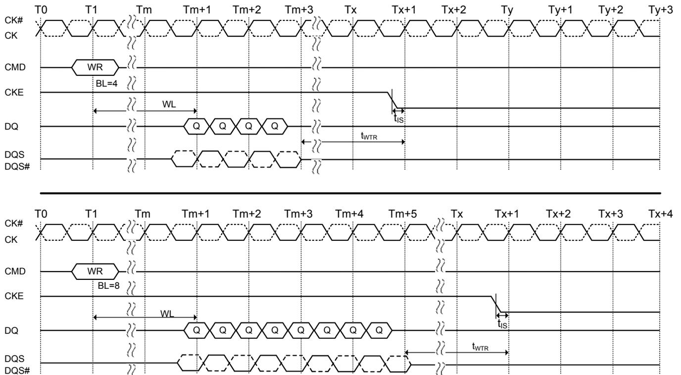
**Figure 51. Write with autoprecharge to power-down entry**
