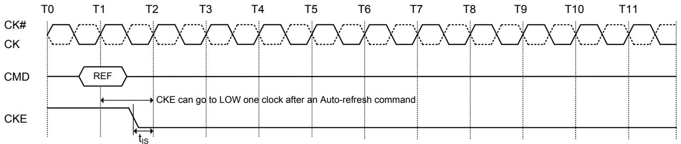
**Figure 53. Active command to power-down entry**
