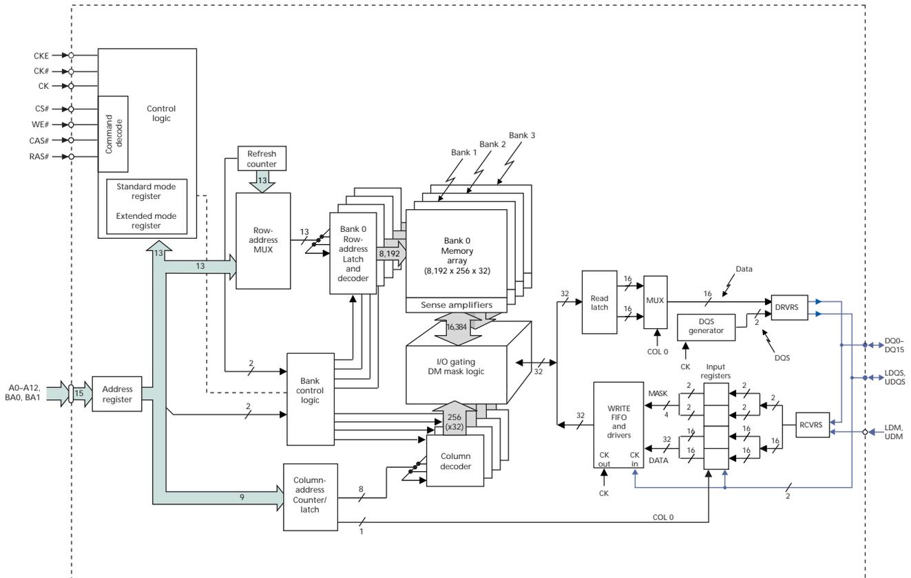
Figure 3: Functional Block Diagram (8 Meg x 32)
