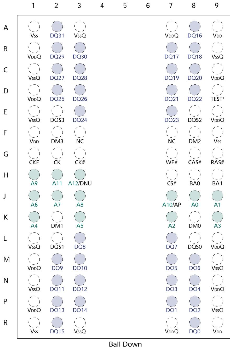
Notes: 1. D9 is a test pin that must be connected to V<sub>SS</sub> or V<sub>SSQ</sub> in normal operation.
