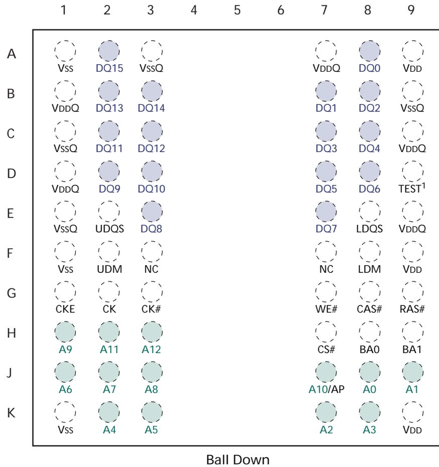
Notes: 1. D9 is a test pin that must be connected to Vss or VssQ in normal operation.
