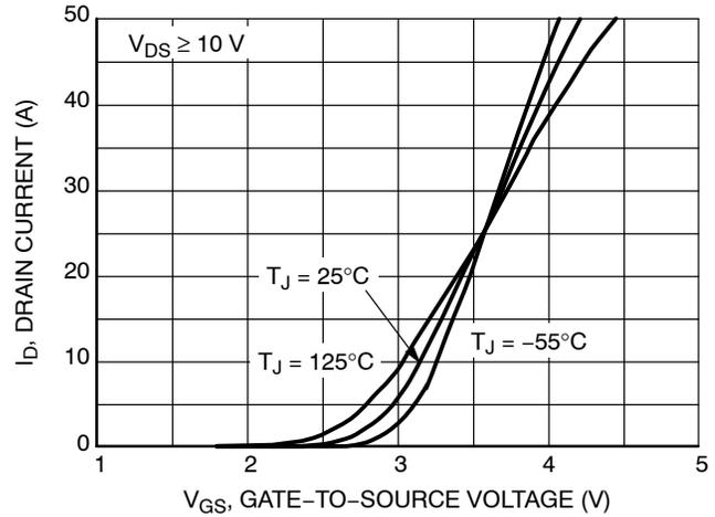
Figure 2. Transfer Characteristics
