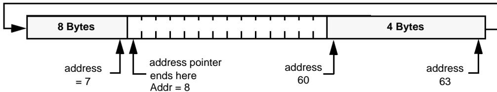
The master terminates the Data Byte loading by issuing a stop condition, which causes the device to begin the nonvolatile write cycle. As with the byte write operation, all inputs are disabled until completion of the internal write cycle. See Figure 9 for the address, acknowledge, and data transfer sequence.
