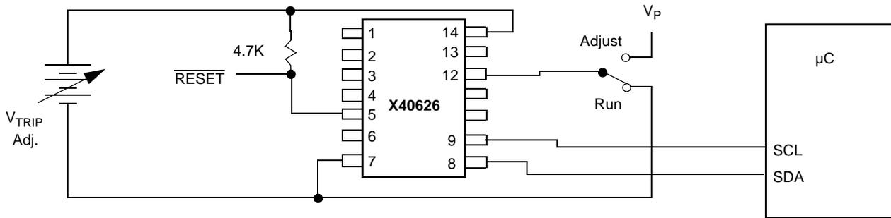
Figure 4.  $V_{TRIPX}$  Programming Sequence
