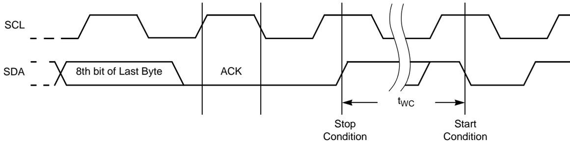
Nonvolatile Write Cycle Timing
