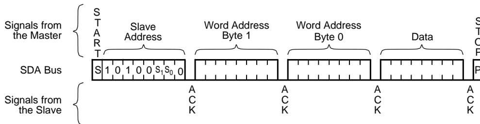
A write to a protected block of memory will suppress the acknowledge bit.
