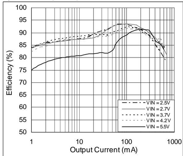
Figure 7. Efficiency vs. Output Current; V<sub>OUT</sub> = 2.5V
