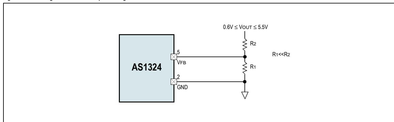
Resistor values for the circuit shown in Figure 27 can be calculated as:
