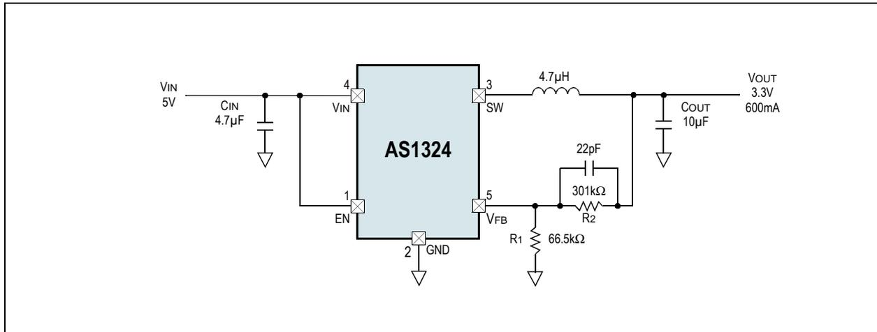
Figure 24. Single Li-Ion 1.5V/600mA Regulator for High-Efficiency
