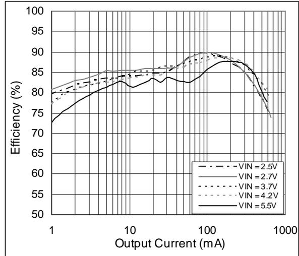
Figure 5. Efficiency vs. Output Current; V<sub>OUT</sub> = 1.5V
