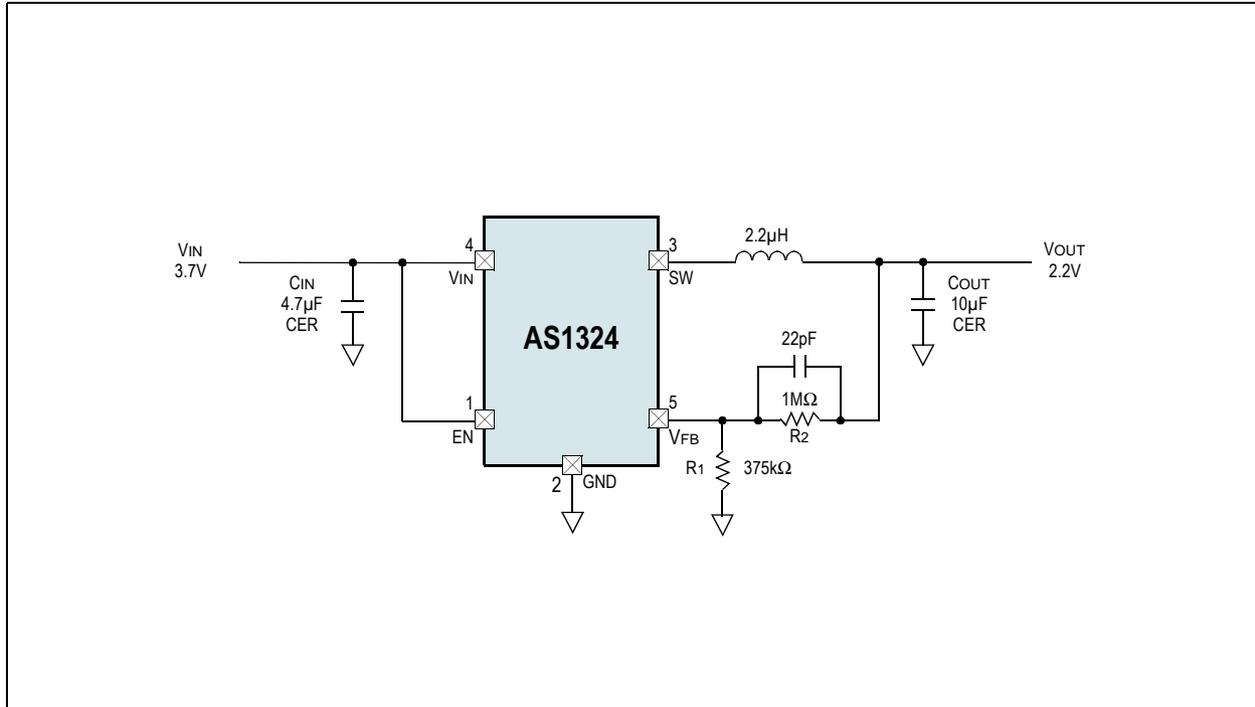
For the circuit shown in Figure 28, efficiency at low- and high-load currents is an important consideration when selecting the value for the external inductor, which is calculated as:
