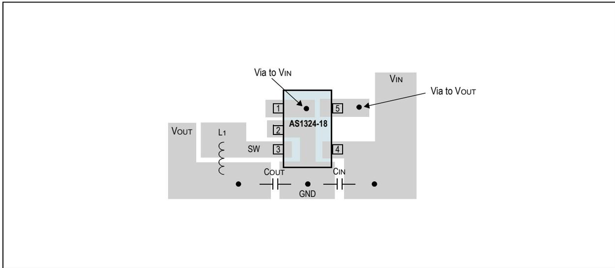
Figure 32. AS1324-18 Basic Diagram
