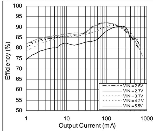
Figure 6. Efficiency vs. Output Current; V<sub>OUT</sub> = 1.8V
