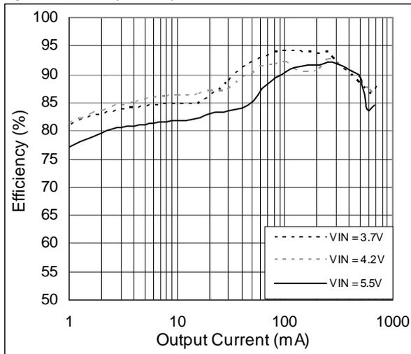
Figure 8. Efficiency vs. Output Current; V<sub>OUT</sub> = 3.3V
