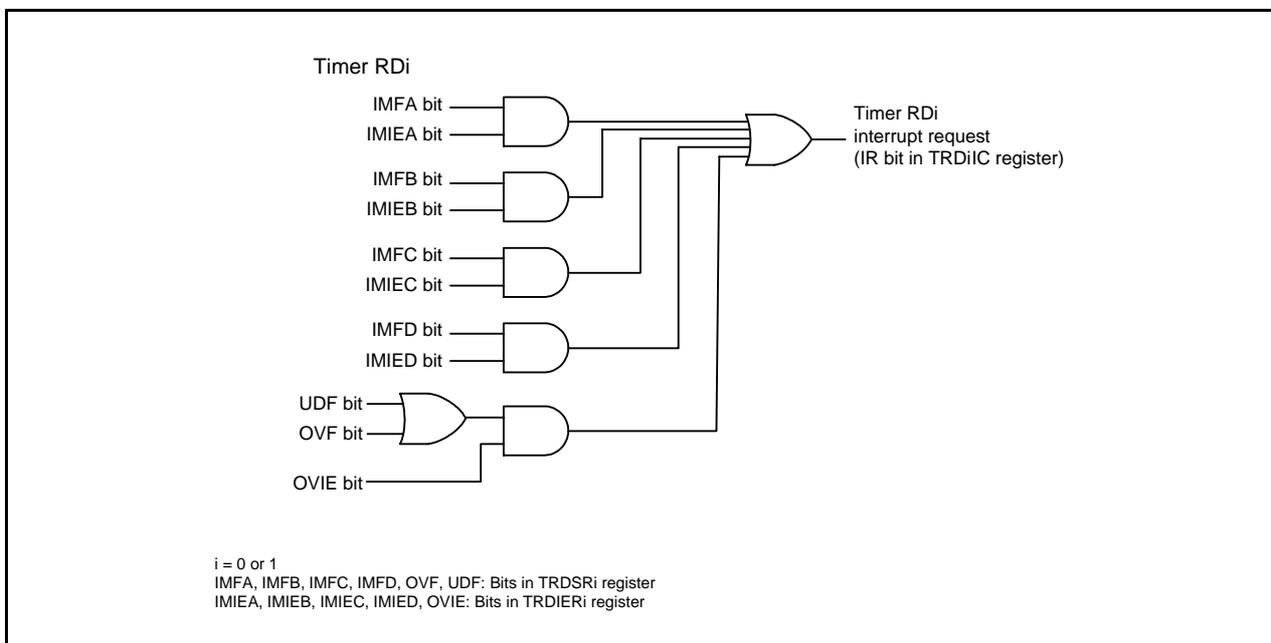
**Figure 11.12 Block Diagram of Timer RD Interrupt**
