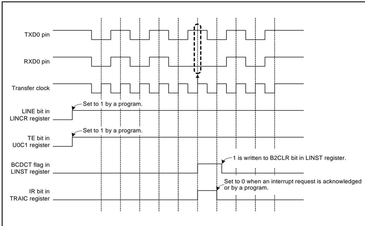
Figure 27.9 Operating Example When Bus Collision is Detected
