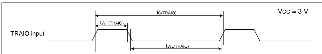
**Figure 33.13 TRAI0 Input Timing Diagram when  $V_{CC} = 3\text{ V}$**
