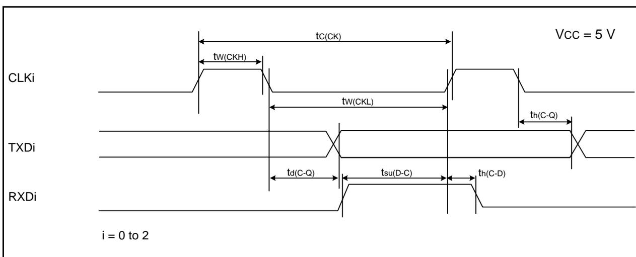
**Figure 33.10 Serial Interface Timing Diagram when Vcc = 5 V**
