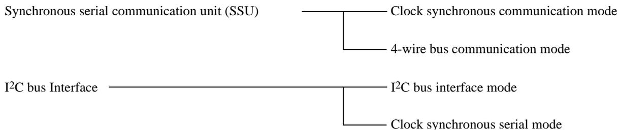
The clock synchronous serial interface uses the registers at addresses 0193h to 019Dh. Registers, bits, symbols, and functions vary even for the same addresses depending on the mode. Refer to the registers of each function for details. Also, the differences between clock synchronous communication mode and clock synchronous serial mode are the options of the transfer clock, clock output format, and data output format.
