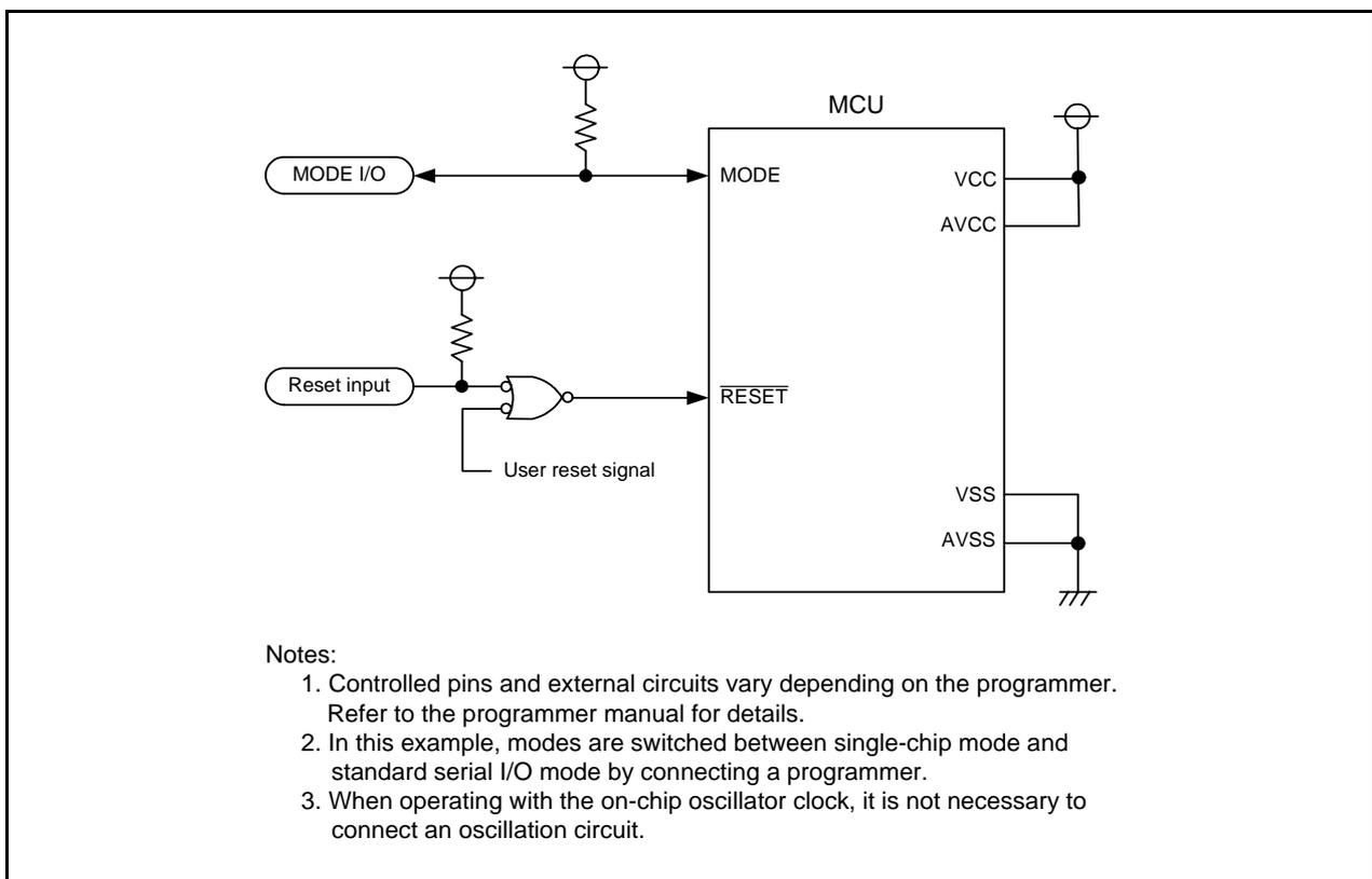
**Figure 31.19 Pin Handling in Standard Serial I/O Mode 3**
