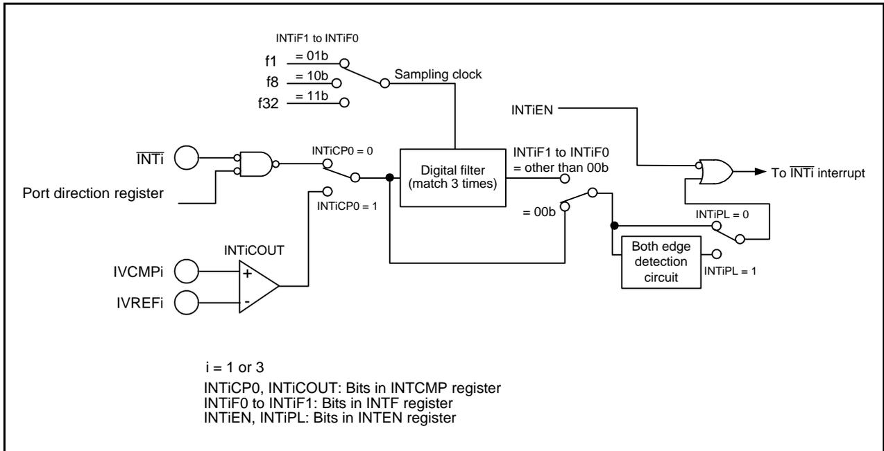
**Figure 30.3 Configuration of Comparator Bi Digital Filter**
