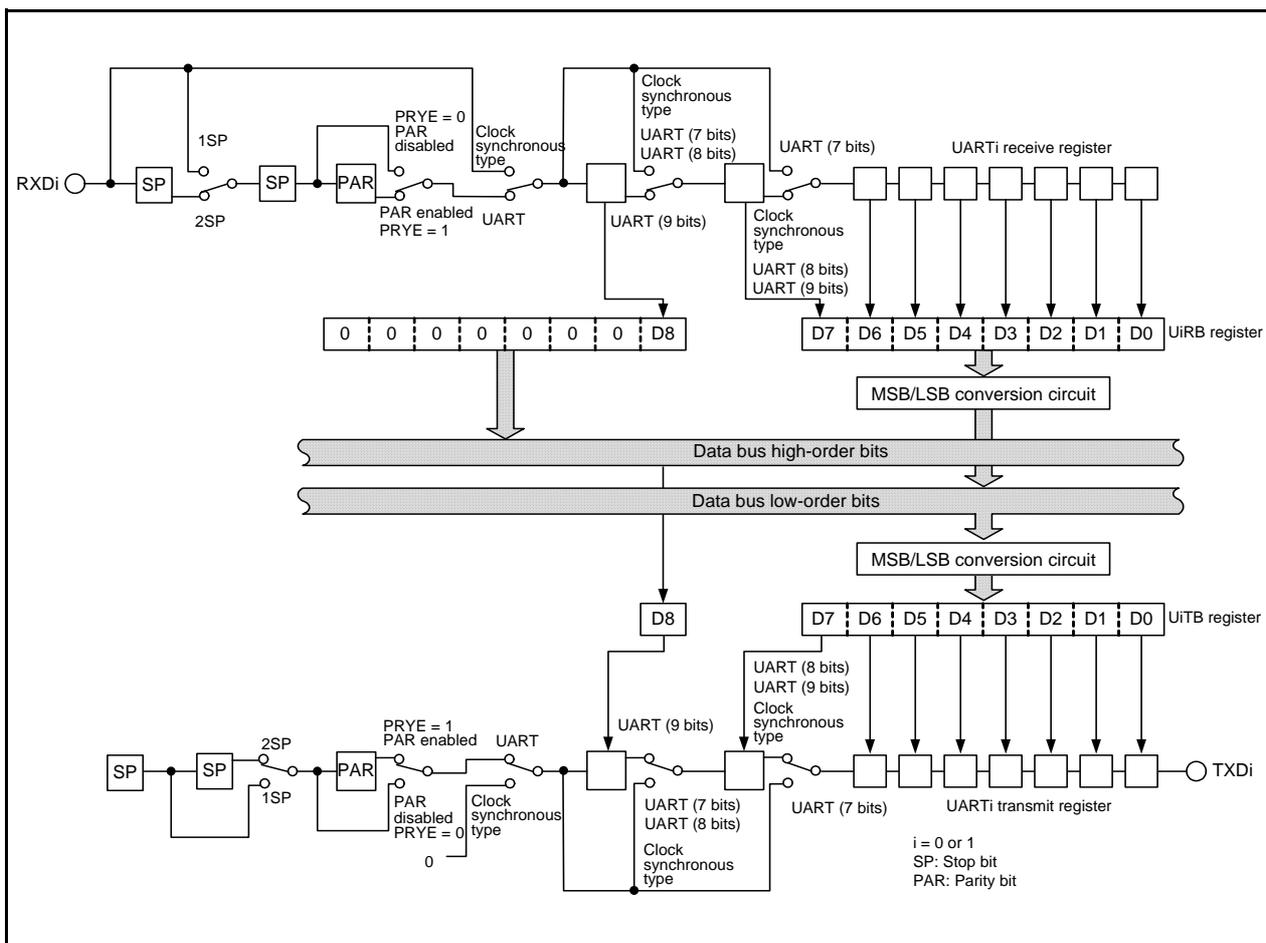
Figure 22.2 Block Diagram of UARTi Transmit/Receive Unit
