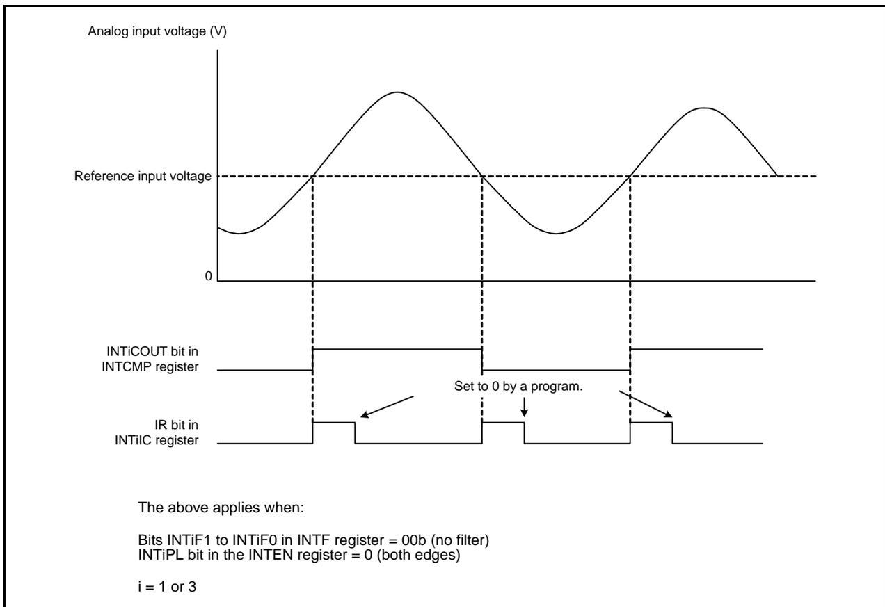
**Figure 30.2 Operating Example of Comparator Bi ( $i = 1$  or  $3$ )**
