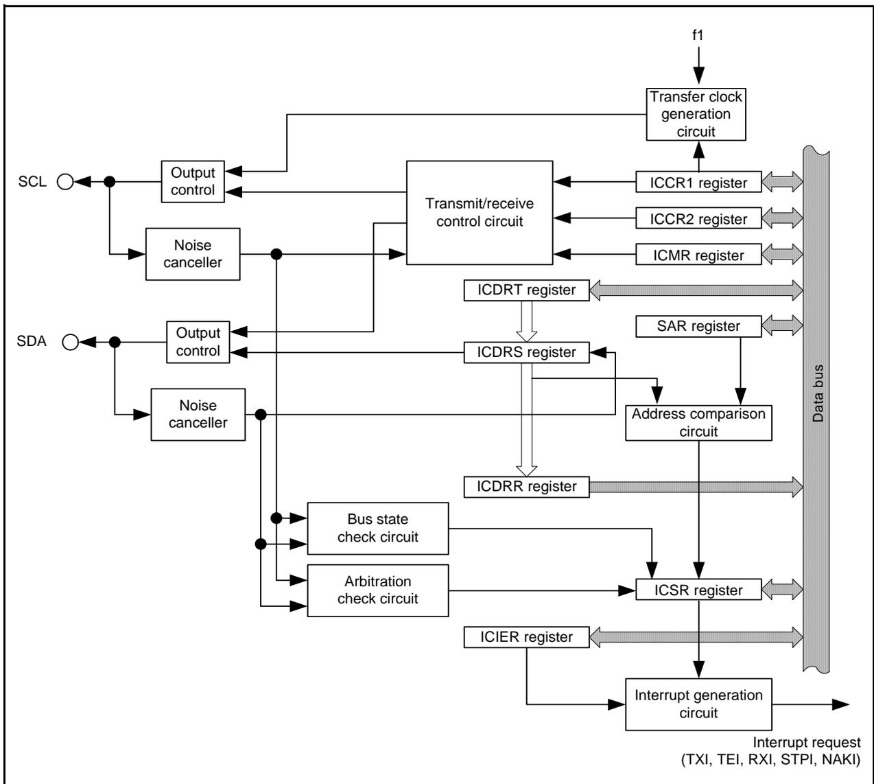
Figure 26.1 I<sup>2</sup>C bus interface Block Diagram
