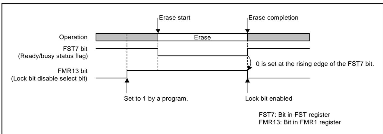
**Figure 31.8 FMR13 Bit Operation Timing**
