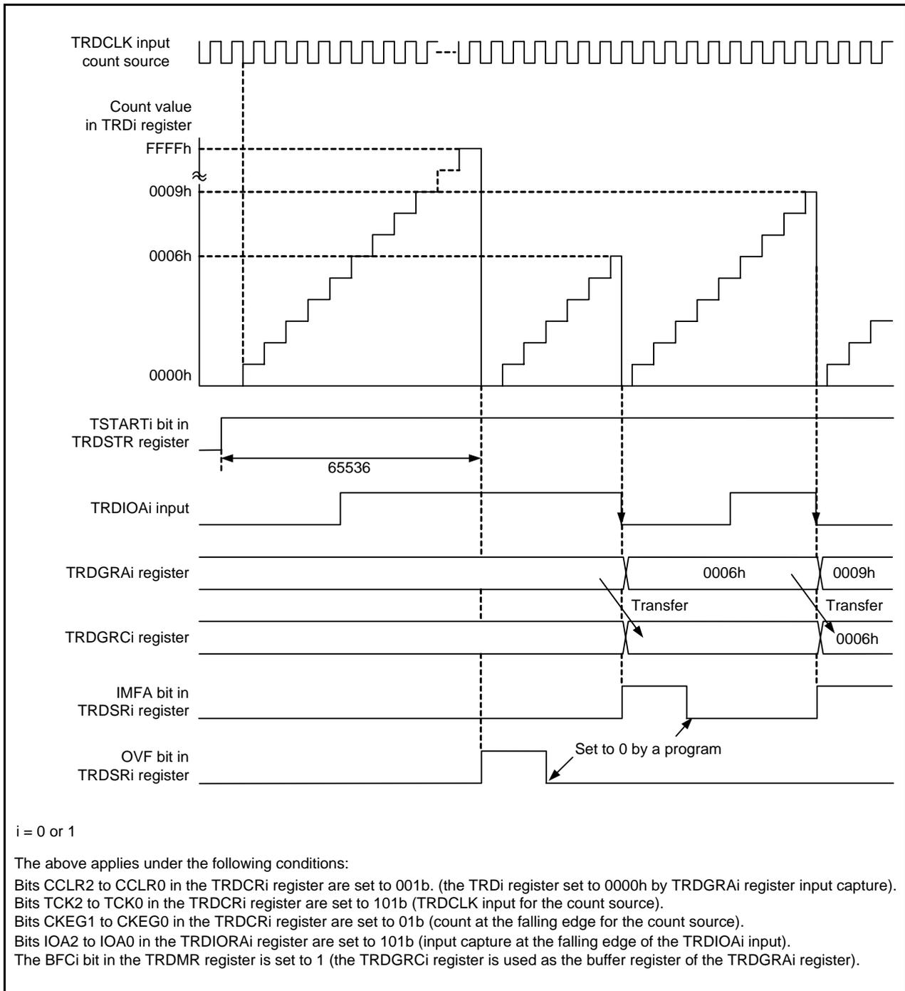
**Figure 20.8** Operating Example of Input Capture Function
