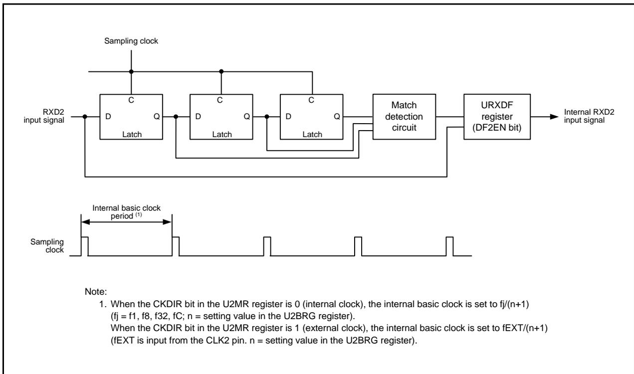
Figure 23.22 Block Diagram of RXD2 Digital Filter Circuit
