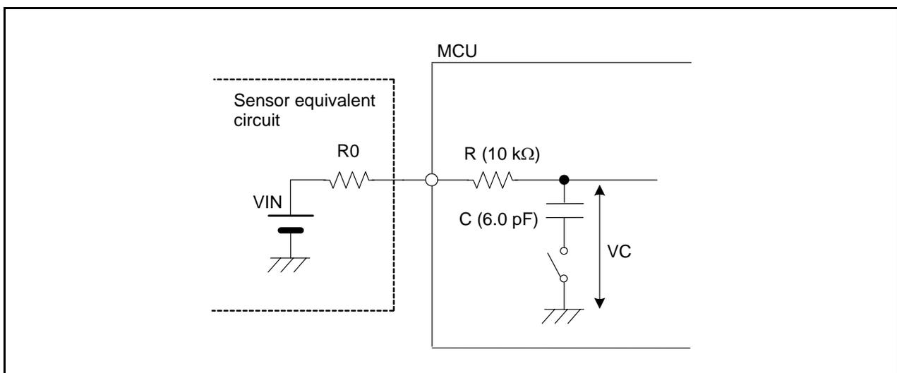
Figure 28.10 Analog Input Pin and External Sensor Equivalent Circuit
