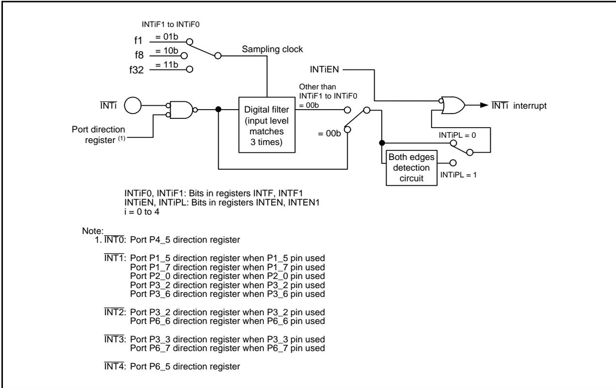
Figure 11.9 INTi Input Filter Configuration
