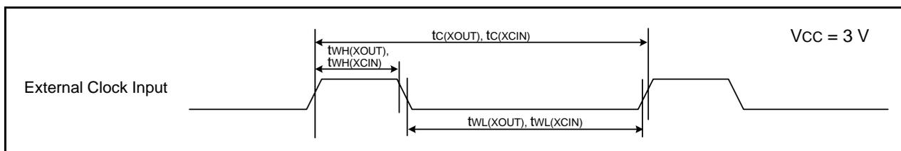
**Figure 33.12 External Clock Input Timing Diagram when  $V_{CC} = 3\text{ V}$** **Table 33.26 TRAI0 Input**
