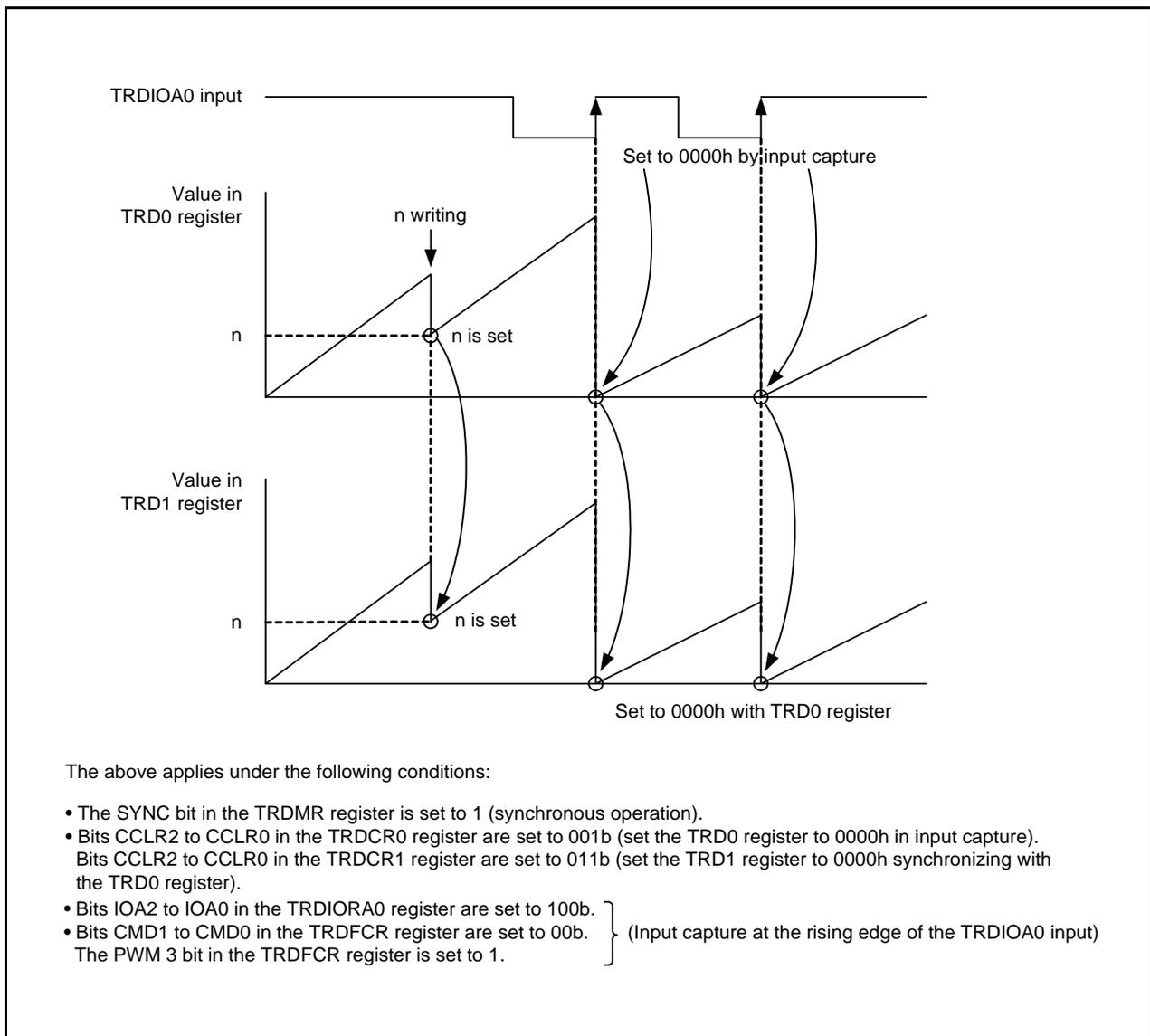
Figure 20.5 Synchronous Operation
