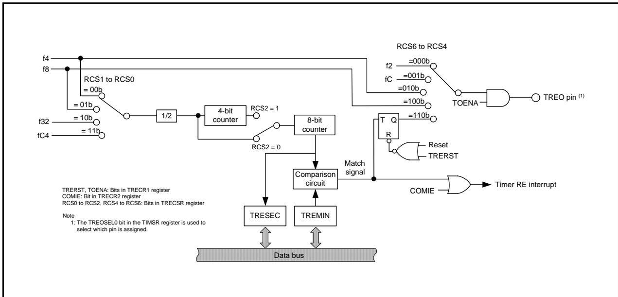
Figure 21.4 Block Diagram of Output Compare Mode
