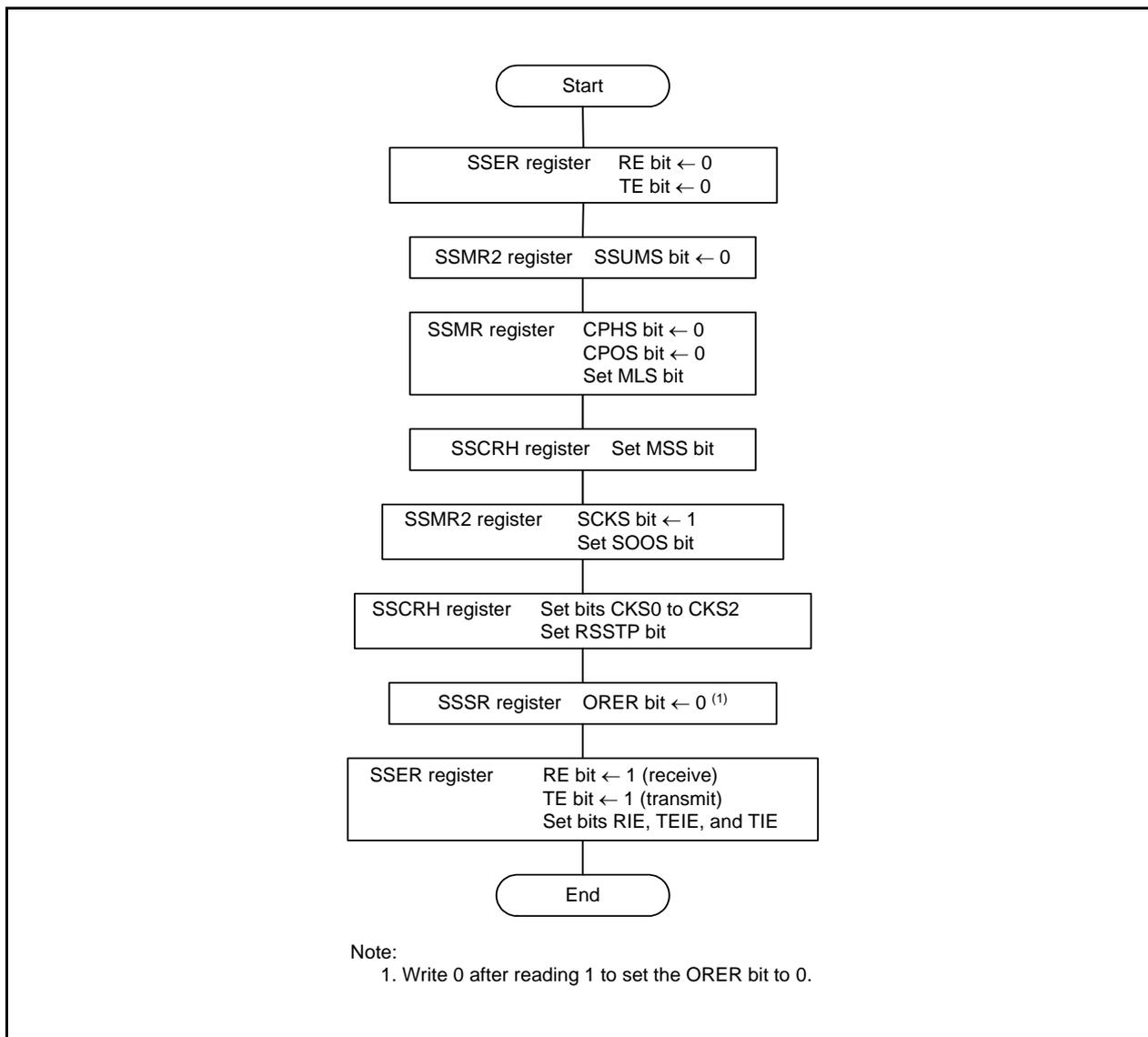
Figure 25.4 Initialization in Clock Synchronous Communication Mode
