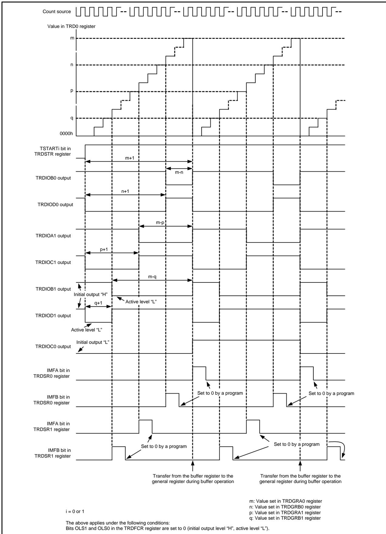
Figure 20.18 Operating Example of Reset Synchronous PWM Mode
