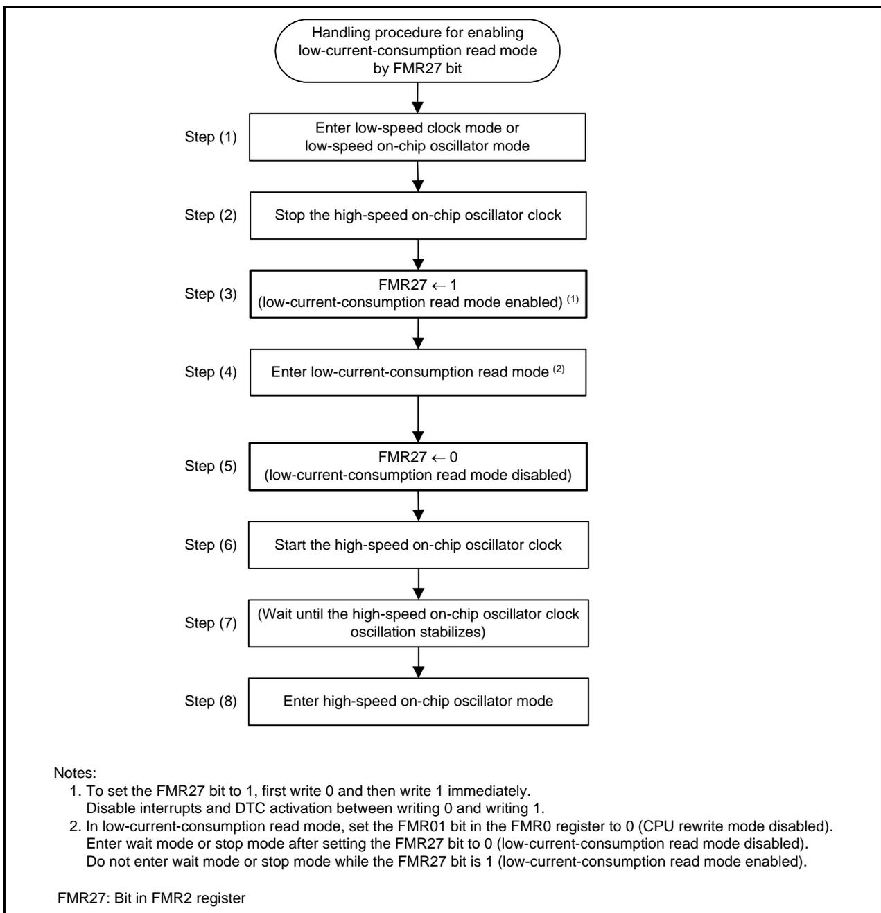
**Figure 32.3 Handling Procedure Example of Low-Current-Consumption Read Mode**
