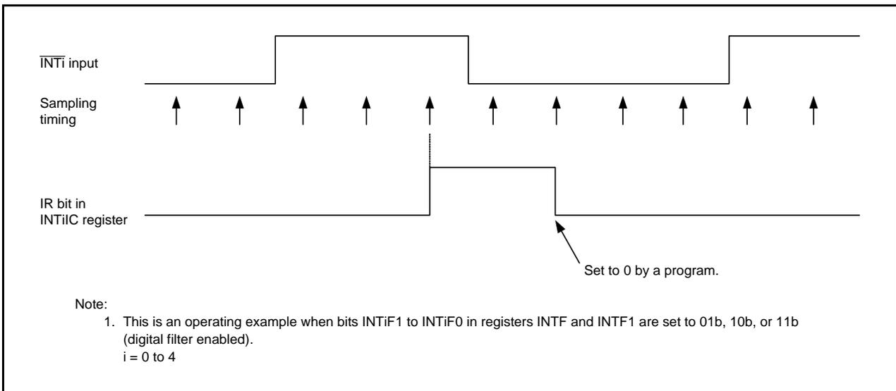
Figure 11.10 Operating Example of INTi Input Filter
