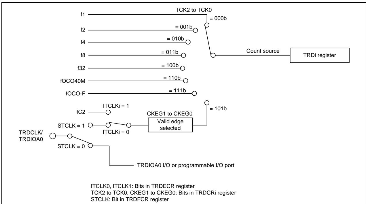
**Figure 20.2 Block Diagram of Count Source**
