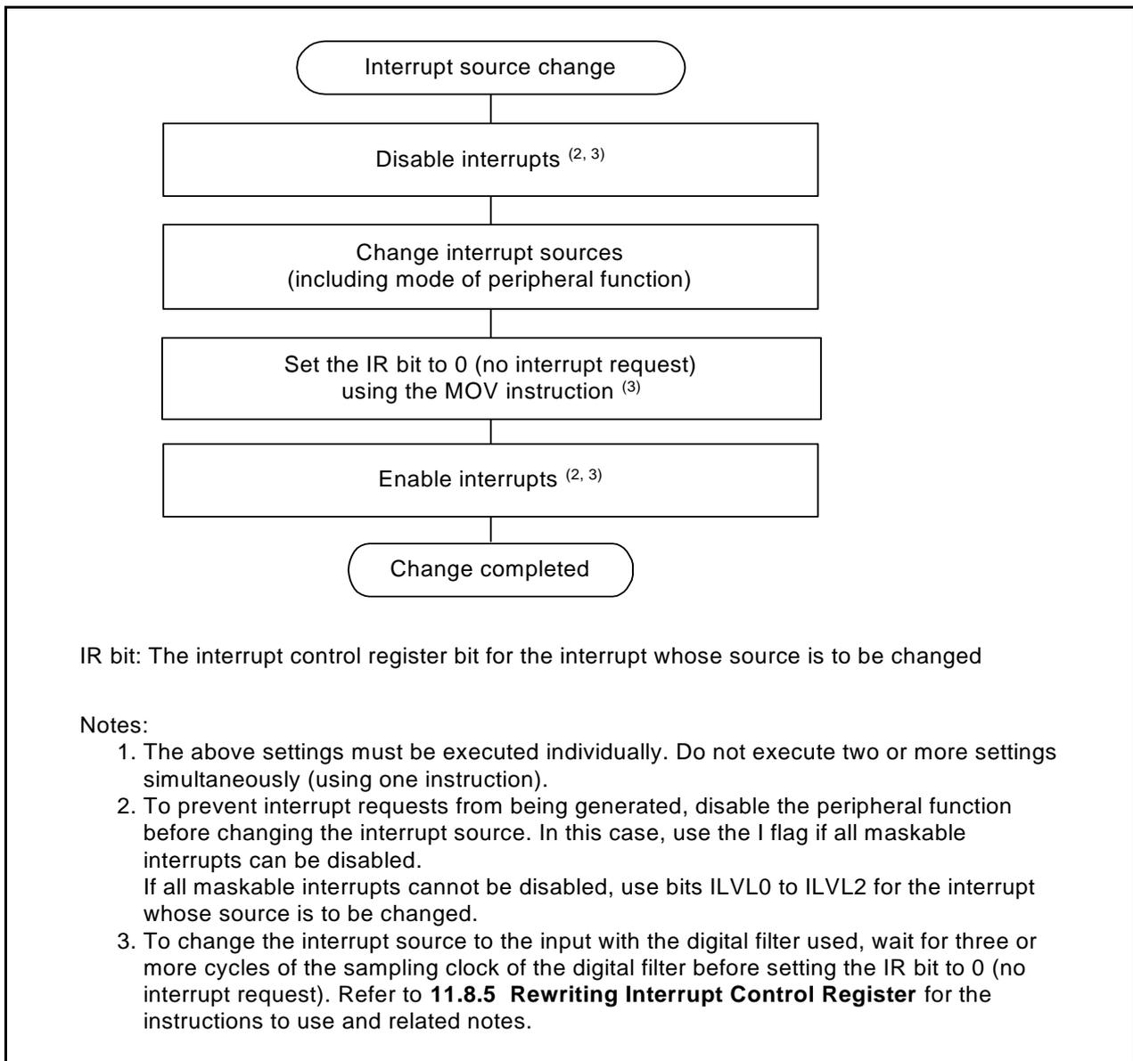
Figure 34.1 Procedure Example for Changing Interrupt Sources
