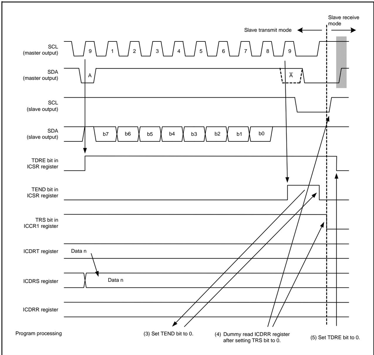
Figure 26.10 Operating Timing in Slave Transmit Mode (I<sup>2</sup>C bus Interface Mode) (2)
