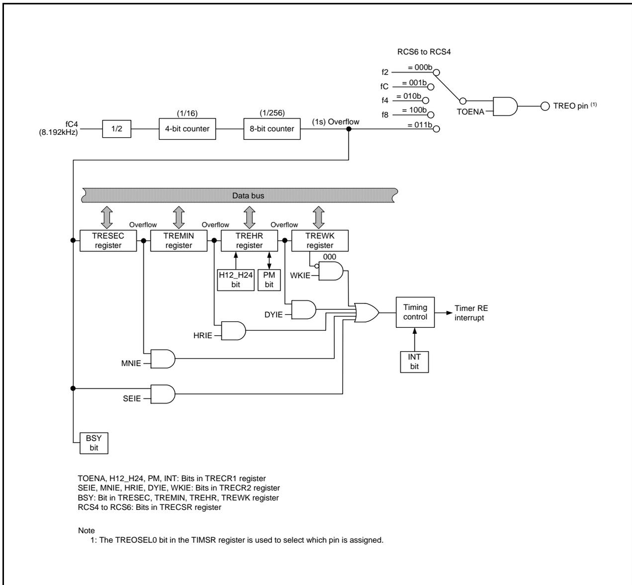
Figure 21.1 Block Diagram of Real-Time Clock Mode
