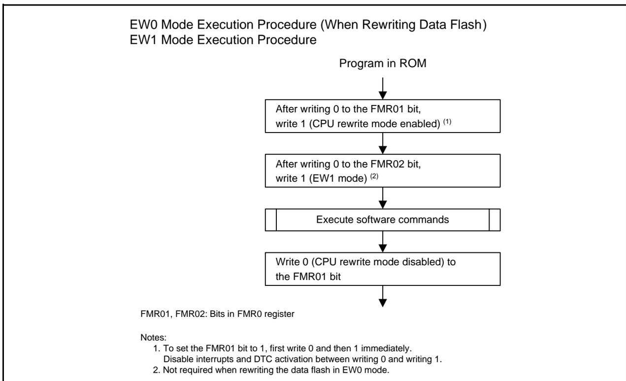
**Figure 31.6 How to Set and Exit EW0 Mode (When Rewriting Data Flash) and EW1 Mode**
