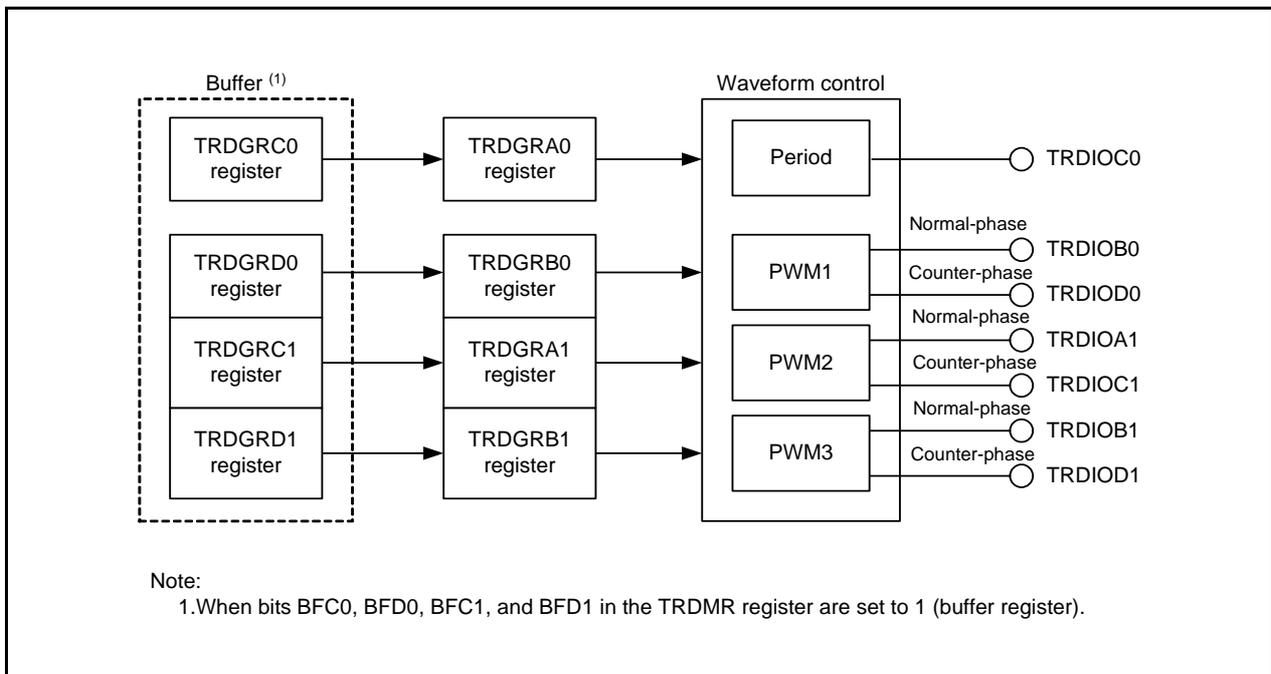
**Figure 20.17 Block Diagram of Reset Synchronous PWM Mode**
