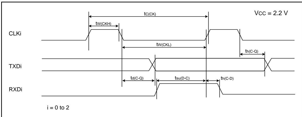
**Figure 33.18 Serial Interface Timing Diagram when Vcc = 2.2 V****Table 33.34 External Interrupt  $\overline{INT}_i$  (i = 0 to 4) Input, Key Input Interrupt  $\overline{K}_i$  (i = 0 to 3)**
