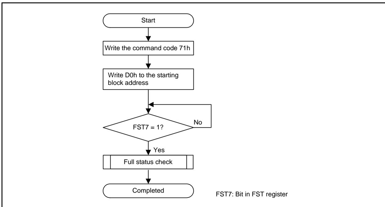
Figure 31.15 Read Lock Bit Status Flowchart
