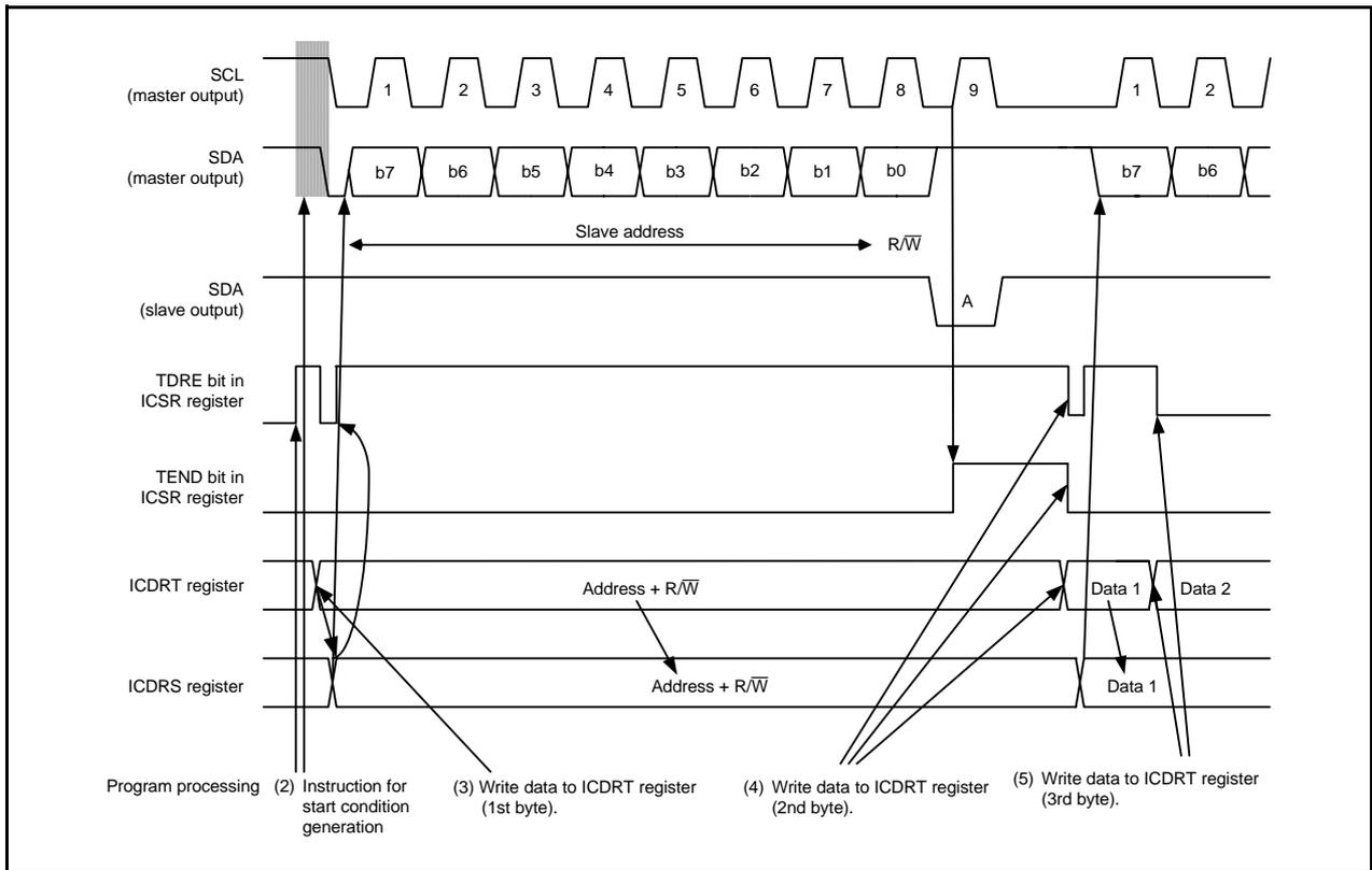
Figure 26.5 Operating Timing in Master Transmit Mode (I<sup>2</sup>C bus Interface Mode) (1)
