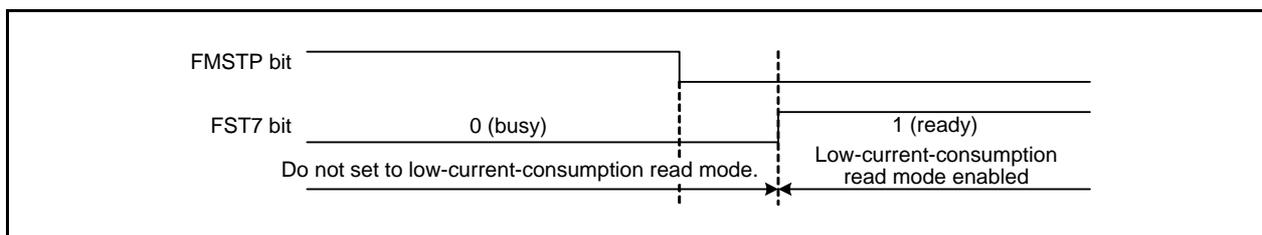
Figure 31.3 Transition to Low-Current-Consumption Read Mode
