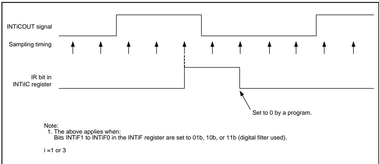
**Figure 30.4 Operating Example of Comparator Bi Digital Filter**
