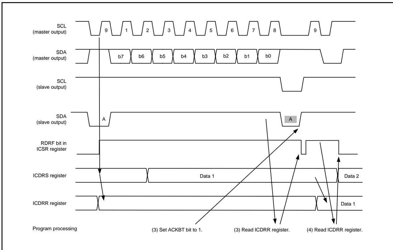
**Figure 26.12 Operating Timing in Slave Receive Mode (I<sup>2</sup>C bus Interface Mode) (2)**
