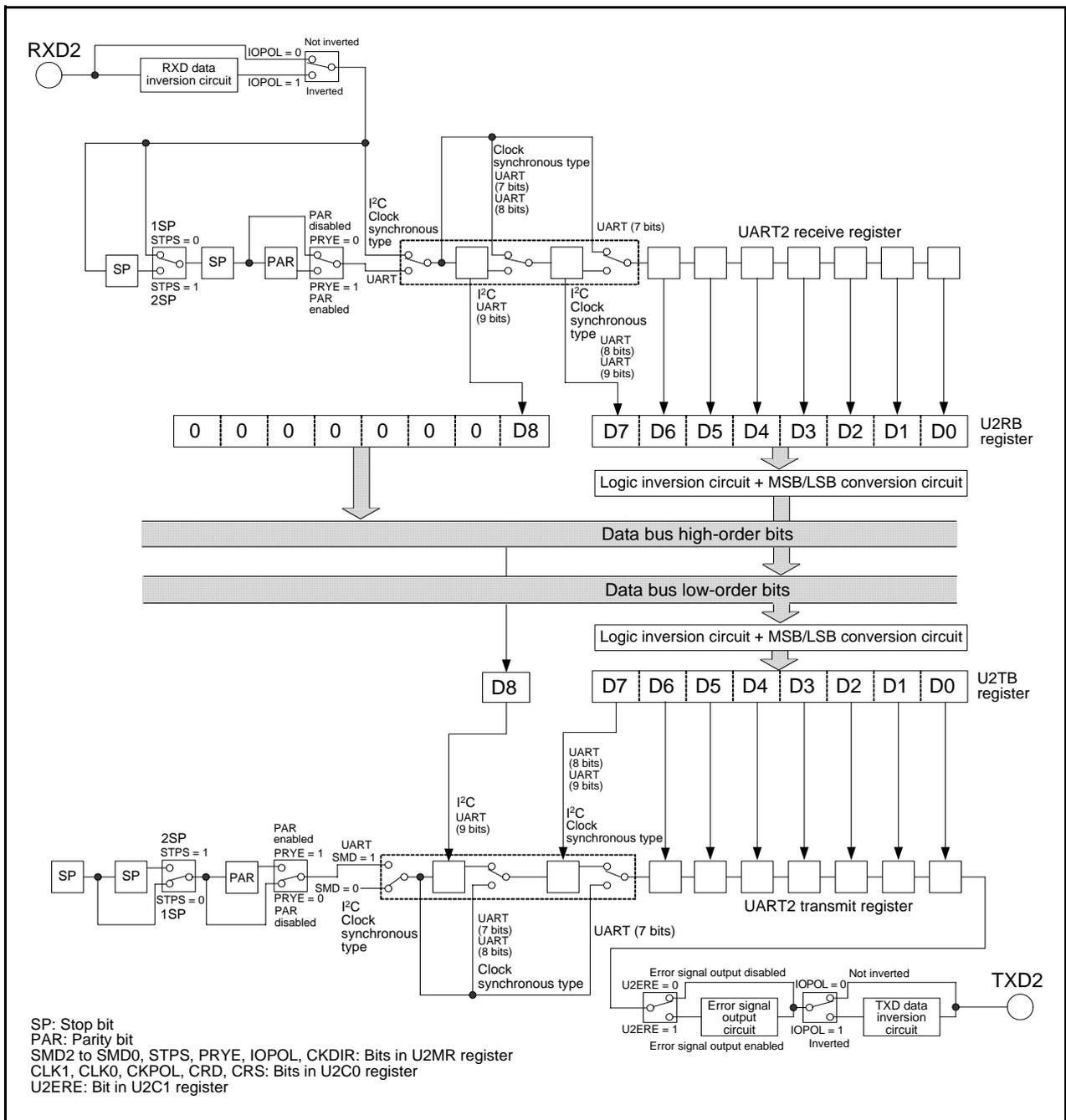
Figure 23.2 Block Diagram of UART2 Transmit/Receive Unit
