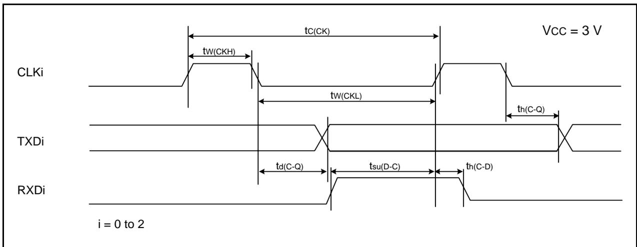
**Figure 33.14 Serial Interface Timing Diagram when Vcc = 3 V**
