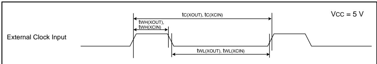
**Figure 33.8 External Clock Input Timing Diagram when  $V_{CC} = 5\text{ V}$** **Table 33.20 TRAIO Input**
