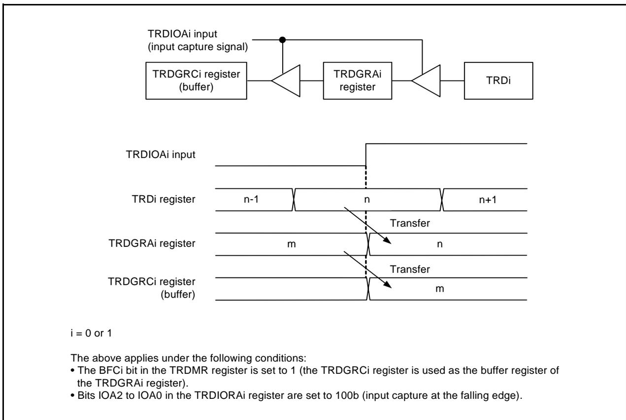
**Figure 20.3 Buffer Operation in Input Capture Function**
