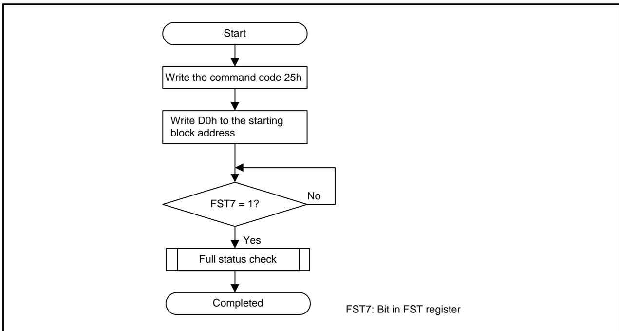
**Figure 31.16 Block Blank Check Flowchart**
