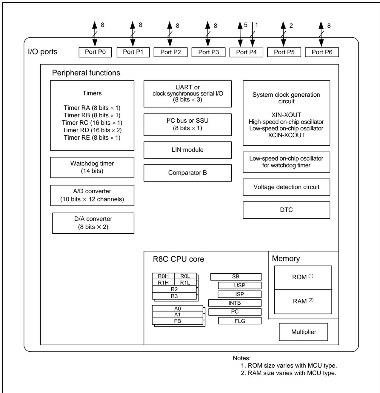
Figure 1.2 Block Diagram
