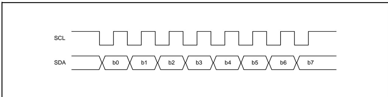
Figure 26.13 Transfer Format of Clock Synchronous Serial Format
