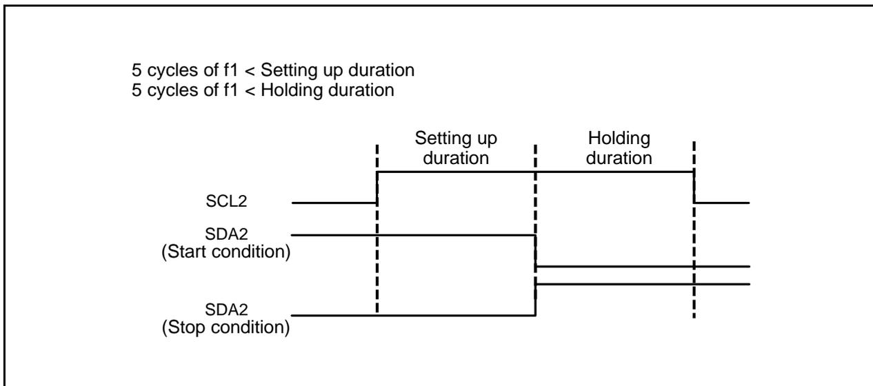
Figure 23.15 Detection of Start and Stop Conditions
