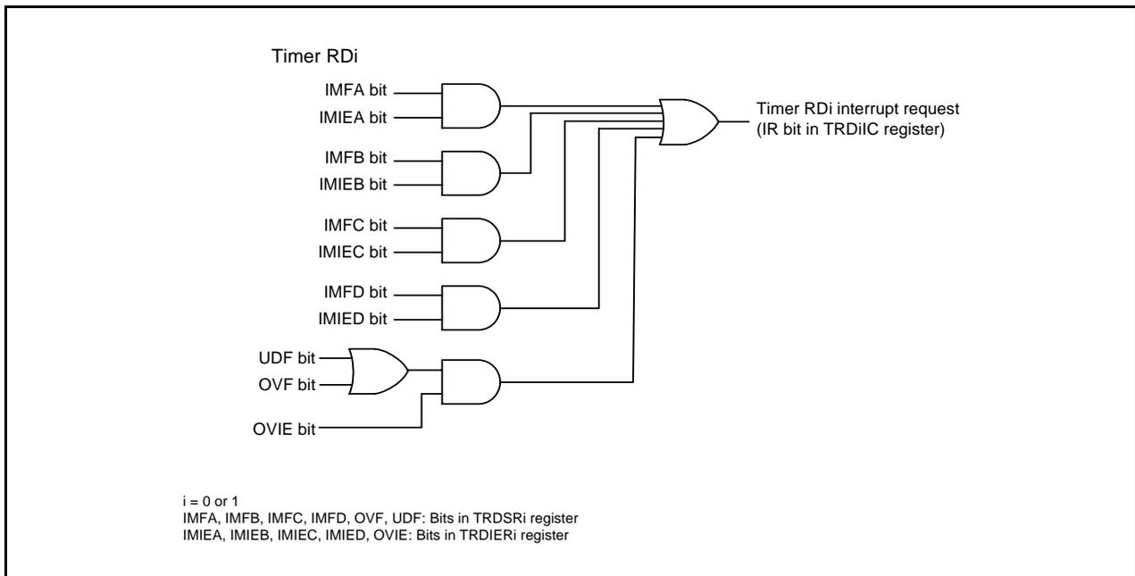
**Figure 20.24 Block Diagram of Timer RD Interrupt**
