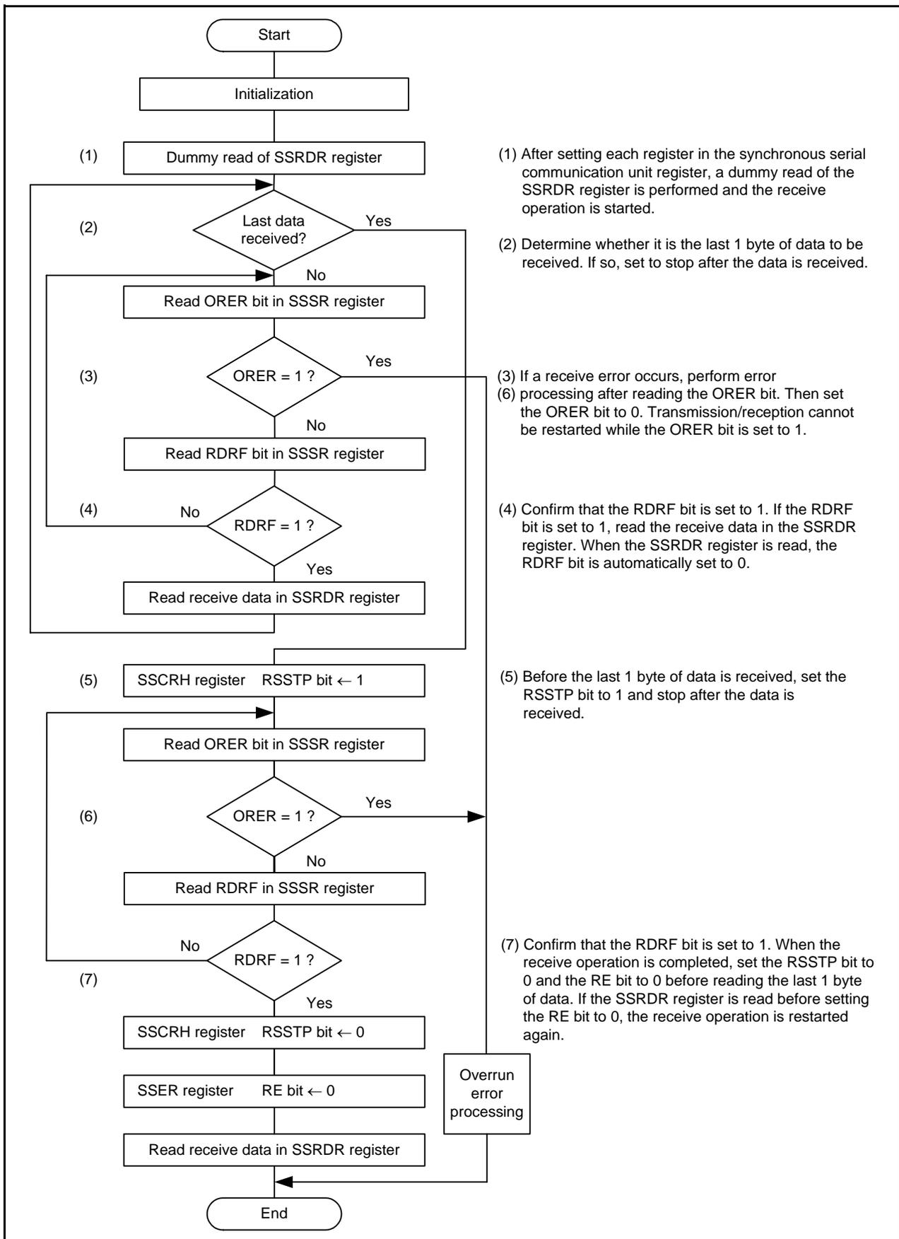
Figure 25.8 Sample Flowchart of Data Reception (MSS = 1) (Clock Synchronous Communication Mode)
