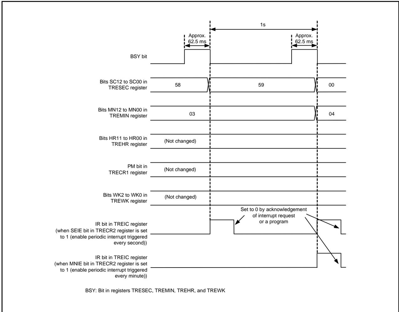
Figure 21.3 Operating Example in Real-Time Clock Mode
