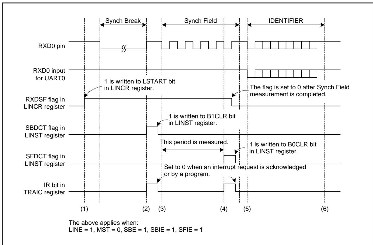
Figure 27.5 Operating Example during Header Field Reception
