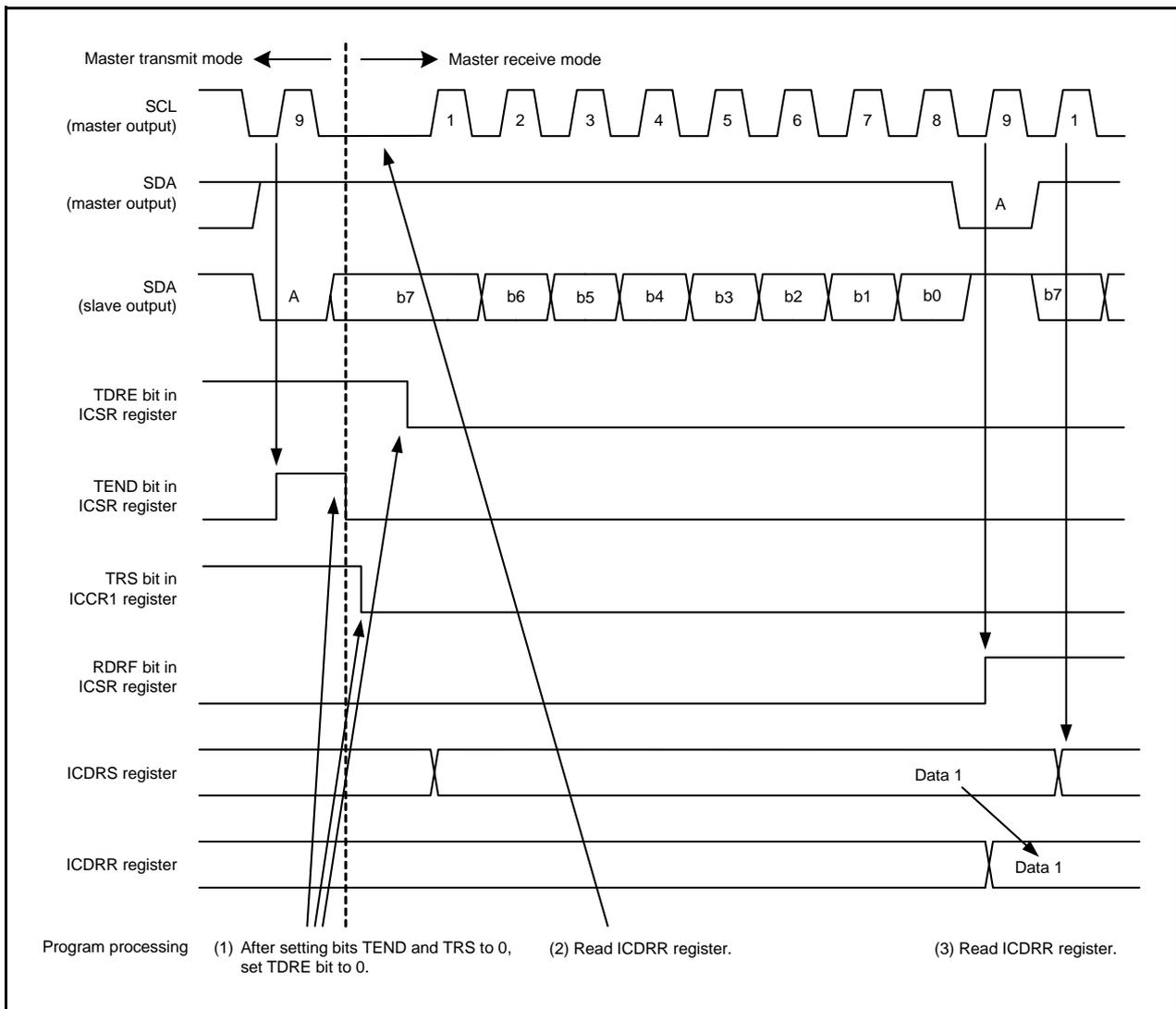
Figure 26.7 Operating Timing in Master Receive Mode (I<sup>2</sup>C bus Interface Mode) (1)
