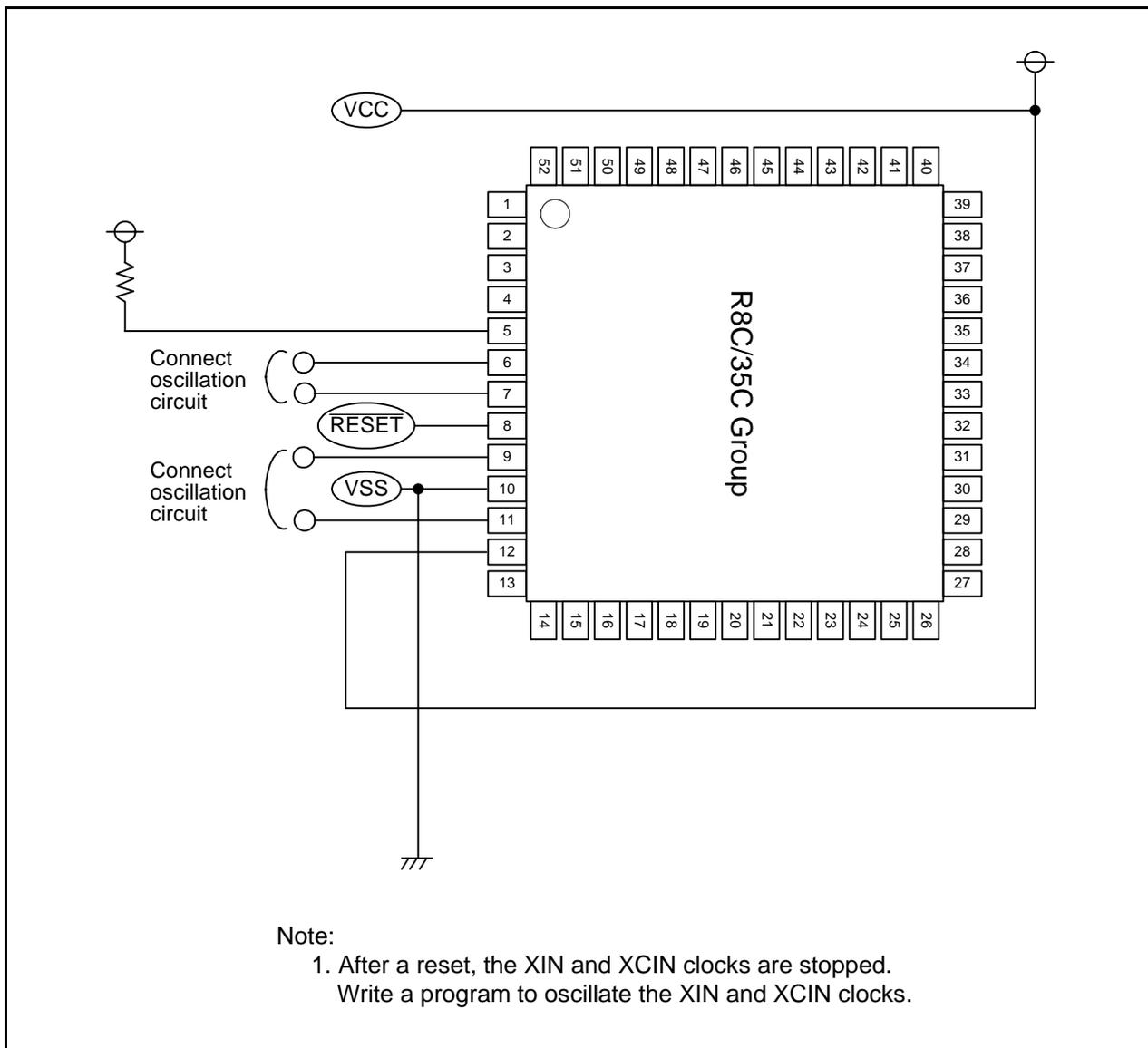
Appendix Figure 3.1 Example of Oscillation Evaluation Circuit
