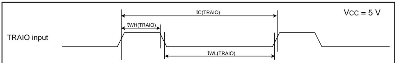
**Figure 33.9 TRAIO Input Timing Diagram when  $V_{CC} = 5\text{ V}$**
