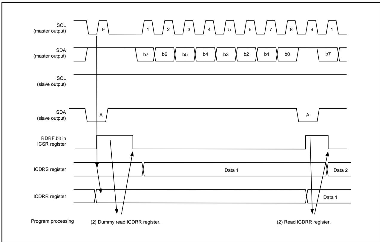
**Figure 26.11 Operating Timing in Slave Receive Mode (I<sup>2</sup>C bus Interface Mode) (1)**
