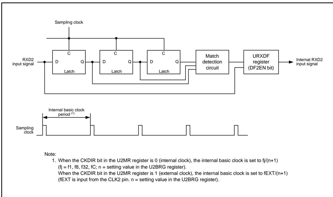
Figure 23.12 Block Diagram of RXD2 Digital Filter Circuit
