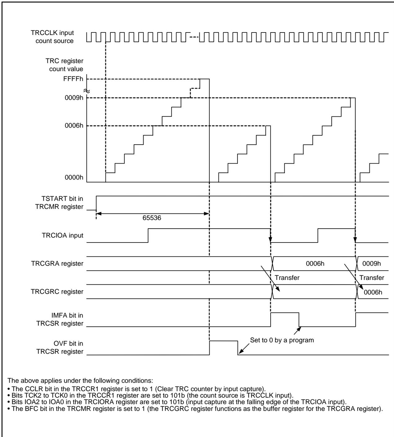
**Figure 19.8** Operating Example of Input Capture Function
