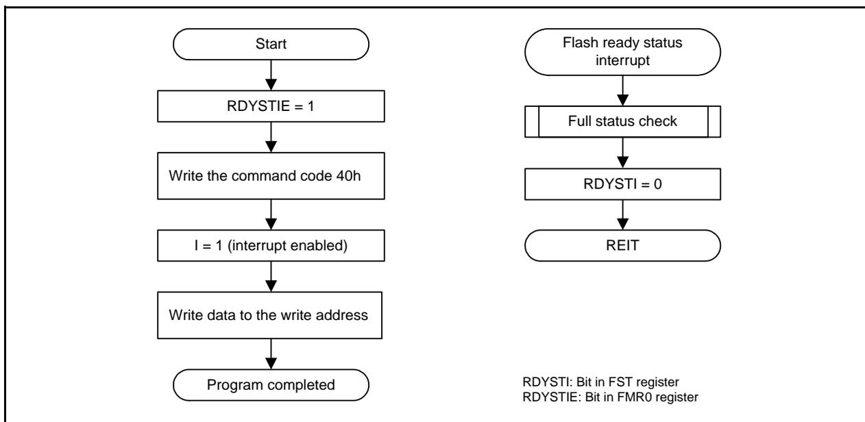
Figure 31.10 Program Flowchart (Flash Ready Status Interrupt Enabled)
