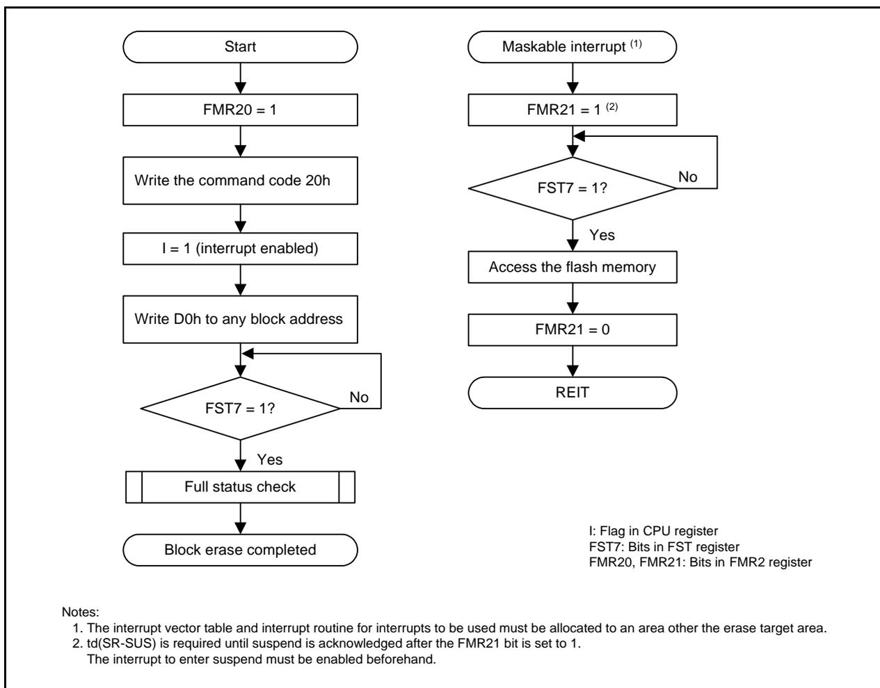
Figure 31.12 Block Erase Flowchart (Flash Ready Status Interrupt Disabled and Suspend Enabled)
