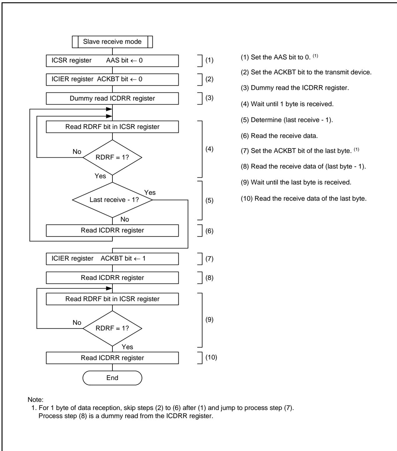
**Figure 26.19 Register Setting Example in Slave Receive Mode (I<sup>2</sup>C bus Interface Mode)**
