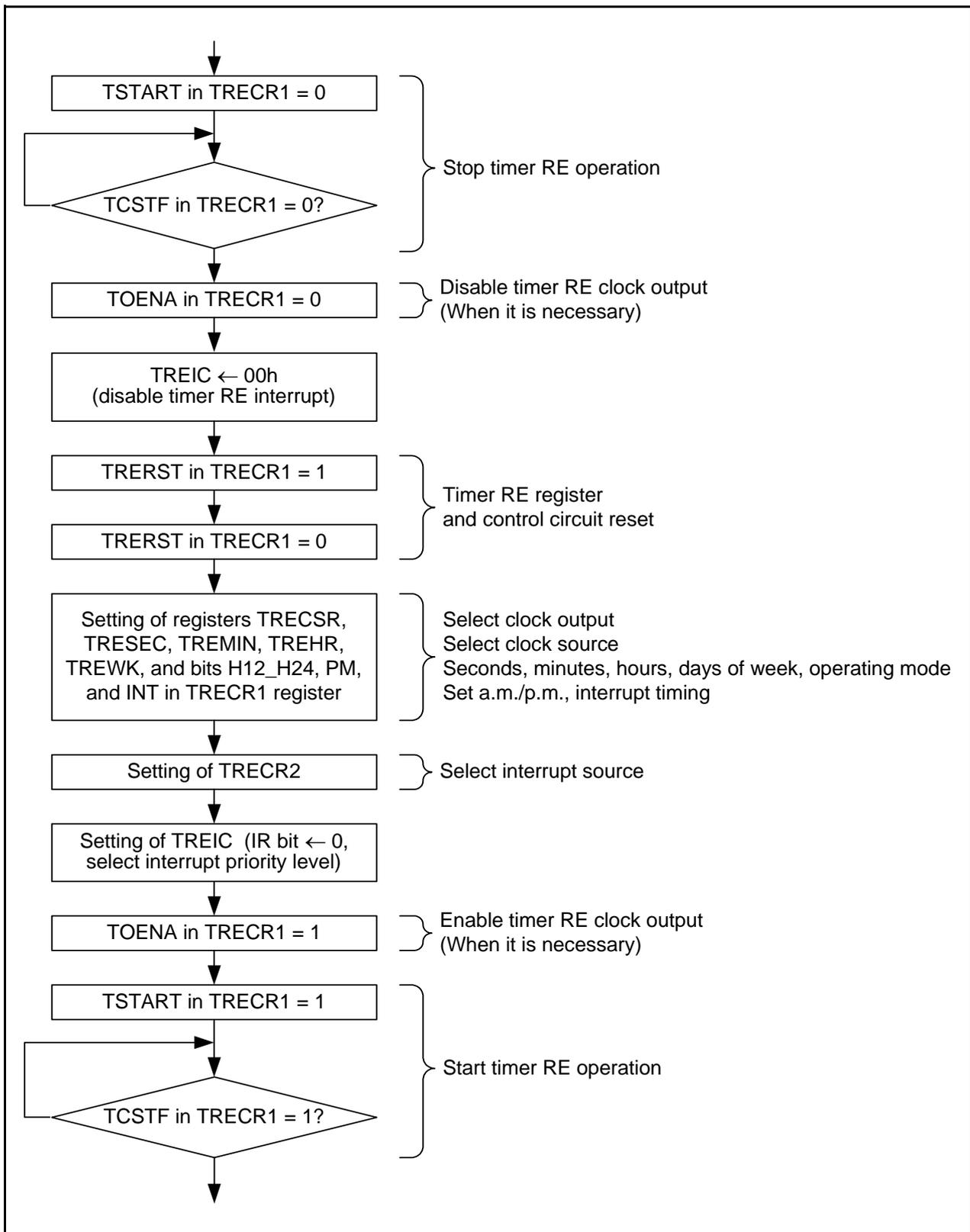
Figure 21.6 Setting Example in Real-Time Clock Mode
