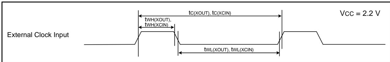
**Figure 33.16 External Clock Input Timing Diagram when  $V_{CC} = 2.2\text{ V}$** **Table 33.32 TRAI0 Input**
