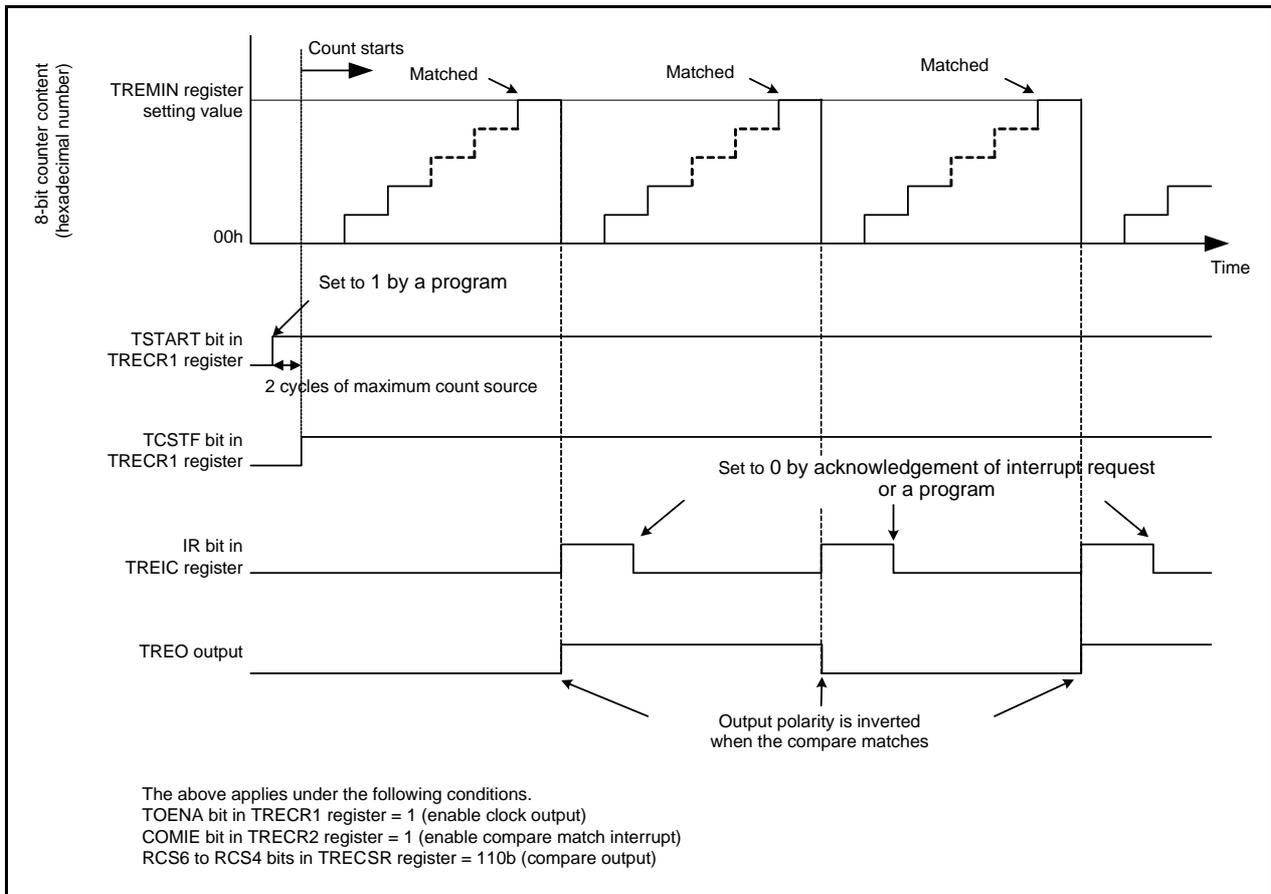
Figure 21.5 Operating Example in Output Compare Mode
