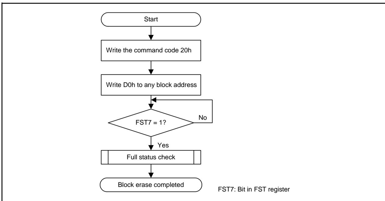
Figure 31.11 Block Erase Flowchart (Flash Ready Status Interrupt Disabled)
