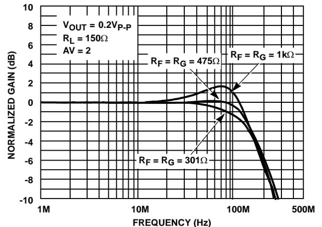
FIGURE 4. SMALL SIGNAL GAIN vs  $R_F$ ,  $R_G$
