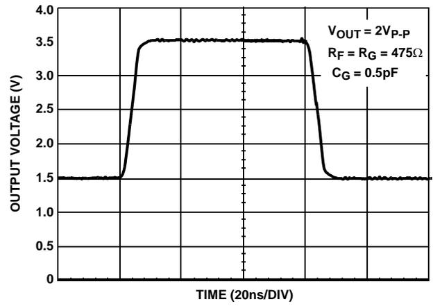
FIGURE 8. LARGE SIGNAL TRANSIENT RESPONSE;  $A_V = 2$
