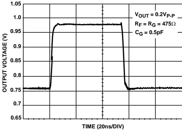
FIGURE 7. SMALL SIGNAL TRANSIENT RESPONSE;  $A_V = 2$
