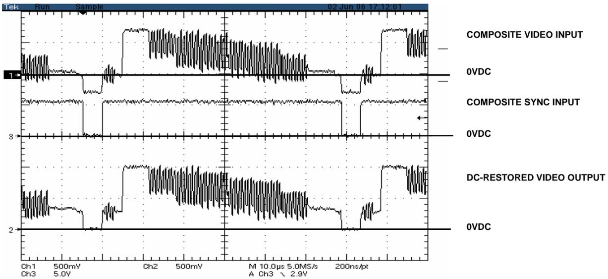
FIGURE 15. DC-RESTORE USING COMPOSITE SYNC AND  $V_{REF} = 0VDC$
