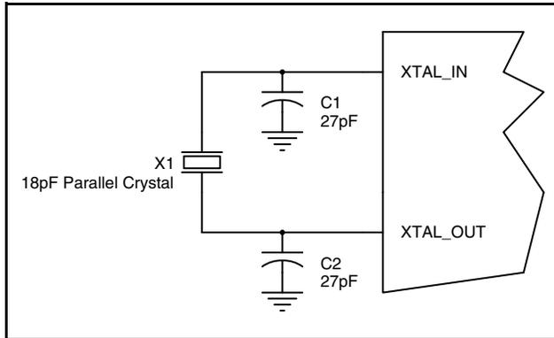
**Figure 2. Crystal Input Interface**
