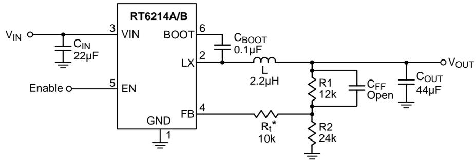
\* Note : When  $C_{FF}$  is added, it is necessary to add  $R_t = 10k$  between feedback network and chip FB pin.
