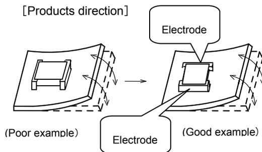
The electrode part of the products should be located like the picture to the mechanical stress.
