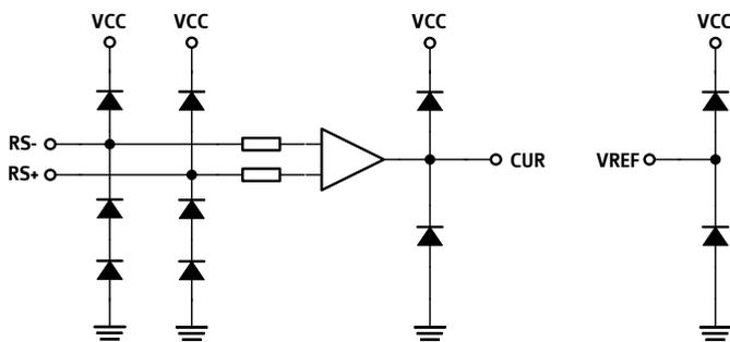
Figure 1.8 Amplifier connections
