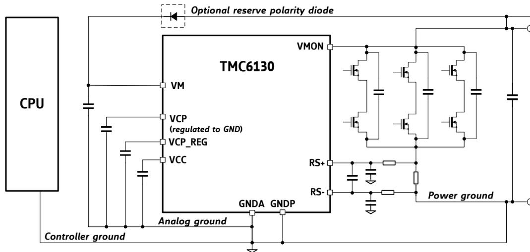
Figure 1.4 Ground connections
