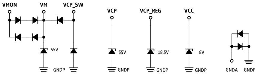
Figure 1.5 Supply connections
