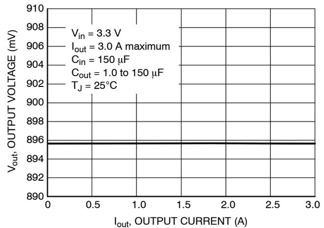
Figure 6. Output Voltage vs. Output Load Current
