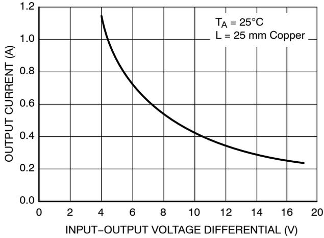
Figure 7. Output Current vs. Input-Output Voltage Differential
