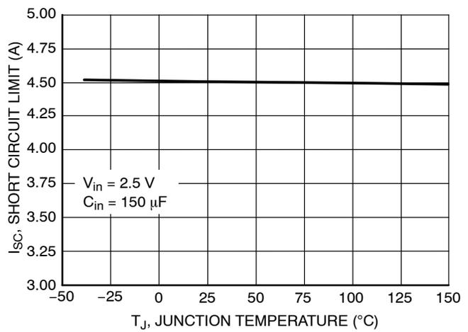
Figure 4. Short Circuit Current Limit vs. Temperature
