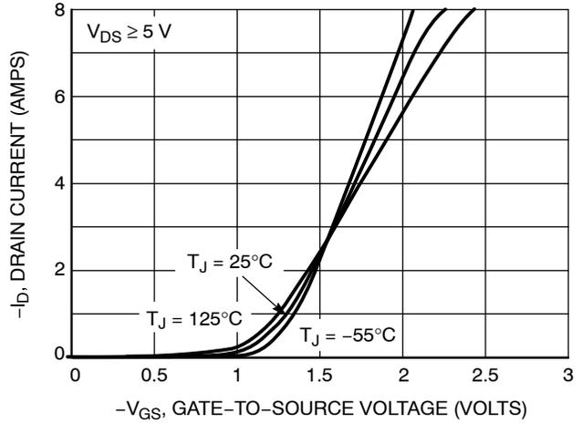
Figure 2. Transfer Characteristics
