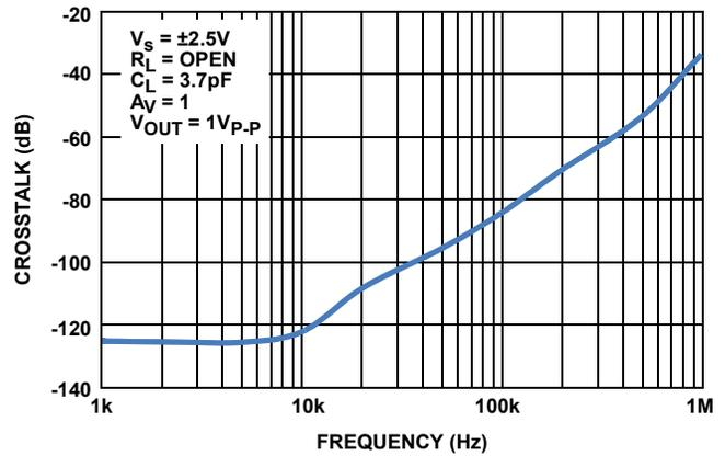
FIGURE 22. CROSSTALK vs FREQUENCY,  $V_S = \pm 2.5V$
