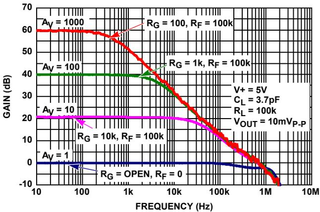
FIGURE 13. FREQUENCY RESPONSE vs CLOSED LOOP GAIN
