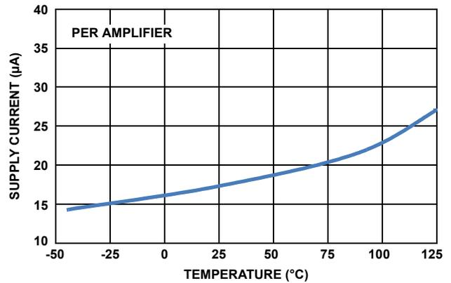
FIGURE 6. SUPPLY CURRENT vs TEMPERATURE,  $V_S = \pm 2.5V$
