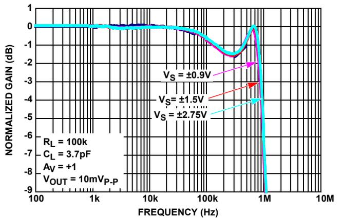
FIGURE 14. GAIN vs FREQUENCY vs SUPPLY VOLTAGE
