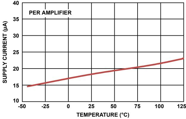
FIGURE 5. SUPPLY CURRENT vs TEMPERATURE,  $V_S = \pm 0.9V$
