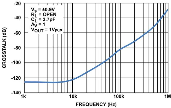
FIGURE 21. CROSSTALK vs FREQUENCY,  $V_S = \pm 0.9V$
