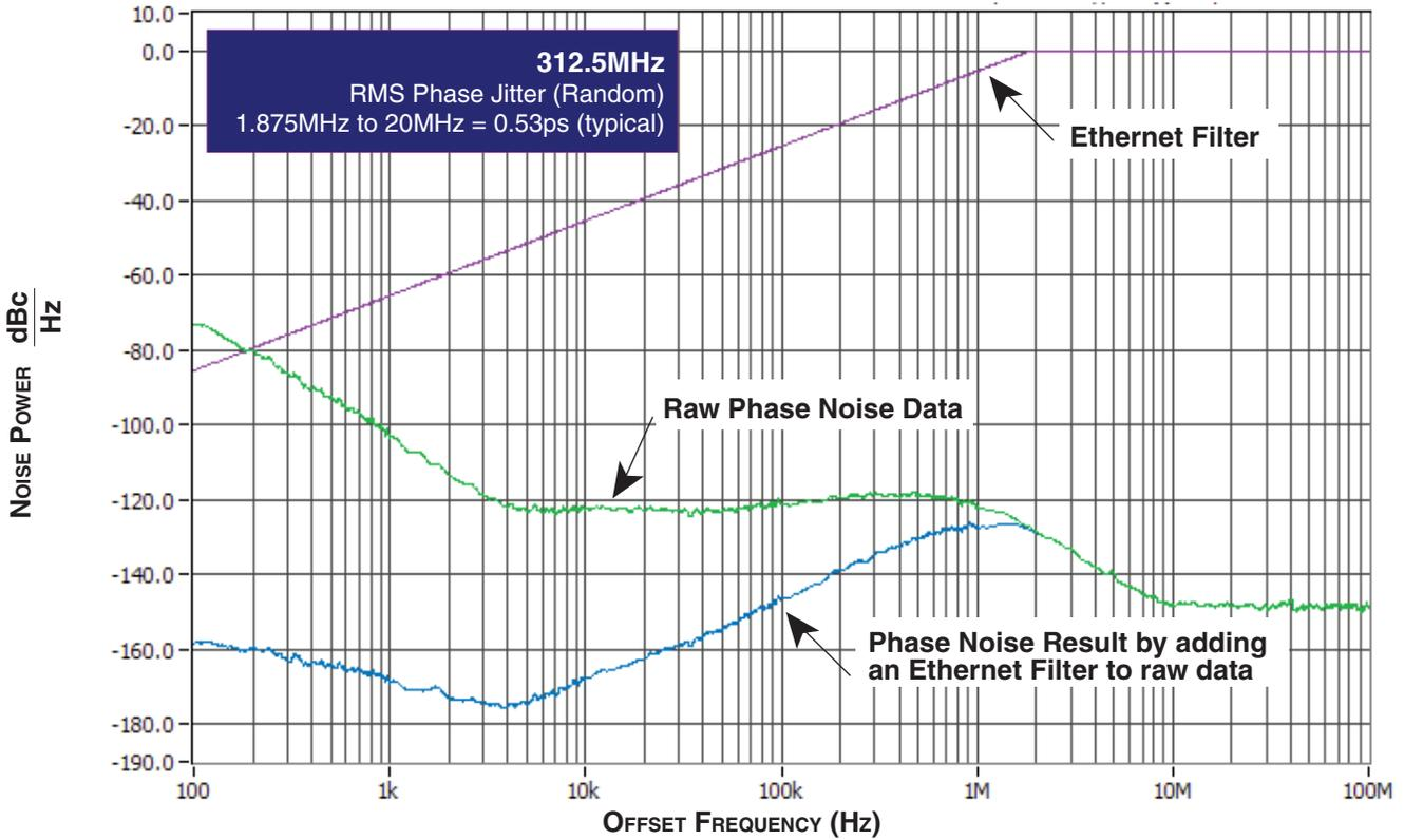
**TYPICAL PHASE NOISE AT 312.5MHz @ 2.5V**
