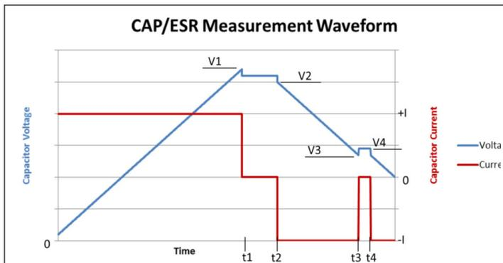
$V1 = V_{\text{rated}}$        $t2 - t1 = 15 \text{ seconds}$        $\text{Capacitance} = I \times (t3-t2)/(V2-V3)$
