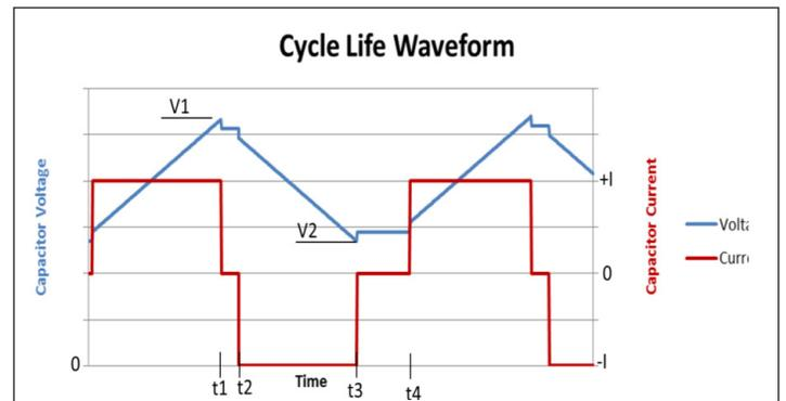
$V1 = V_{\text{rated}}$        $t2 - t1 = 5 \text{ seconds (I=0)}$
