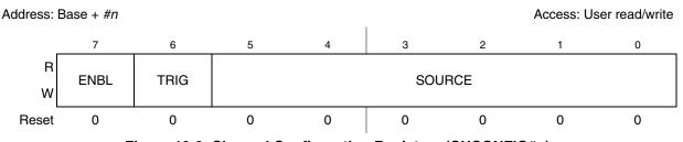
Figure 19-2. Channel Configuration Registers (CHCONFIG#n)
