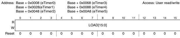
Figure 27-7. Load register (LOAD)
