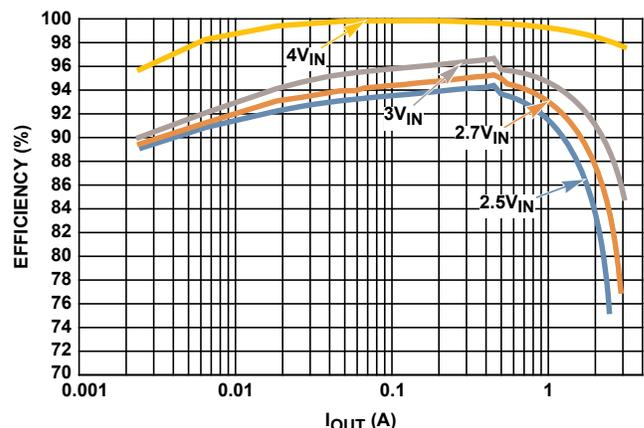
FIGURE 2. EFFICIENCY vs LOAD CURRENT,  $V_{OUT} = 3.3V$
