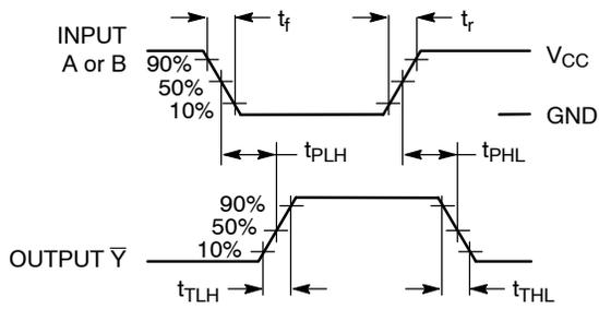
Figure 4. Switching Waveforms
