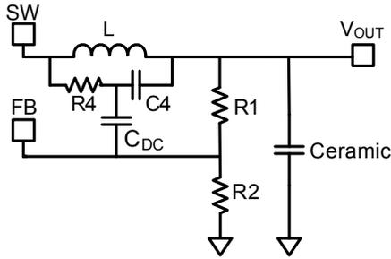
**Figure 9: Simplified Ceramic Capacitor Circuit with DC-Blocking Capacitor**
