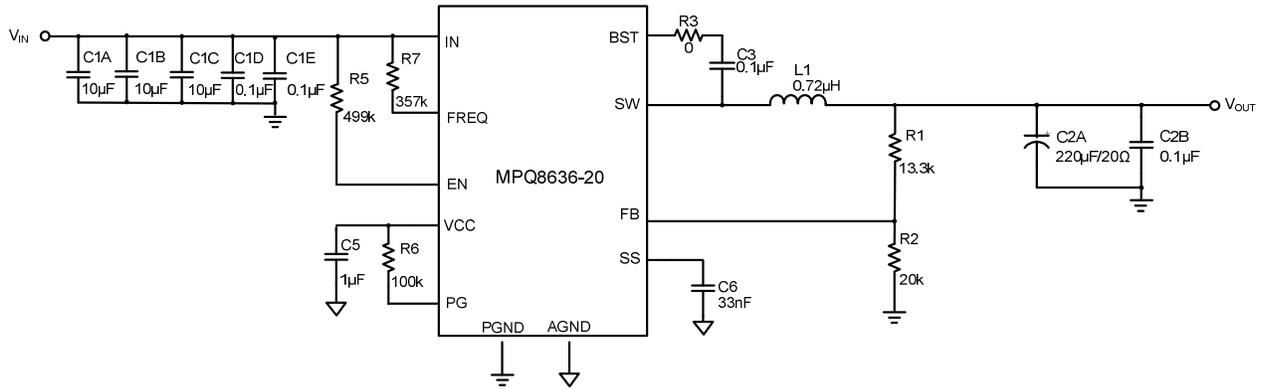
**Figure 10 — Typical Application Circuit with No External Ramp**
