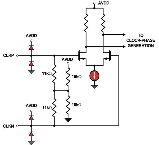
FIGURE 59. CLOCK INPUTS
