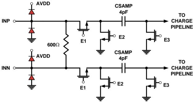
FIGURE 58. ANALOG INPUTS
