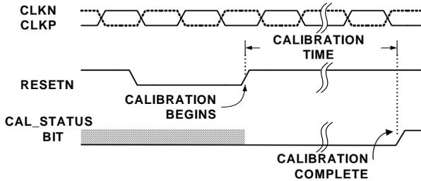
FIGURE 35. CALIBRATION TIMING
