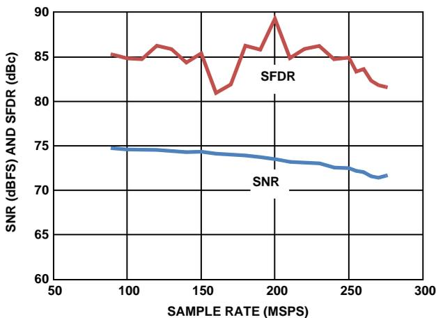
FIGURE 7. SNR AND SFDR vs f<sub>SAMPLE</sub>
