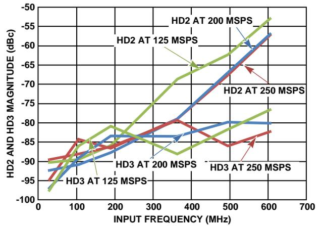
FIGURE 4. HD2 AND HD3 vs f<sub>IN</sub>
