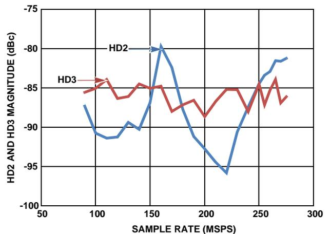
FIGURE 8. HD2 AND HD3 vs f<sub>SAMPLE</sub>
