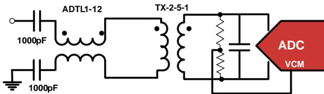
FIGURE 44. TRANSMISSION-LINE TRANSFORMER INPUT FOR HIGH IF APPLICATIONS
