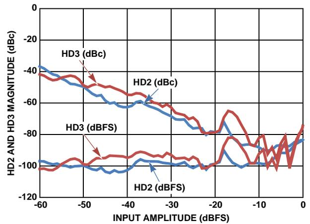
FIGURE 6. HD2 AND HD3 vs A<sub>IN</sub> (250MSPS)
