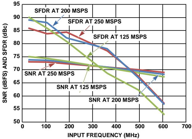
FIGURE 3. SNR AND SFDR vs f<sub>IN</sub>
