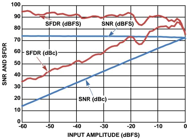
FIGURE 5. SNR AND SFDR vs A<sub>IN</sub> (250MSPS)
