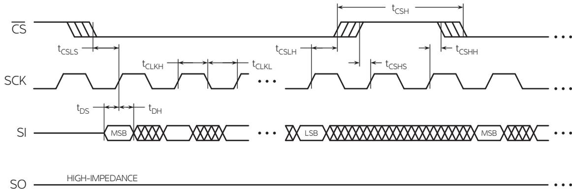
Figure 14-2. Serial output timing
