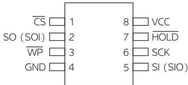
Figure 2-2. 8-UDFN (Top View)
