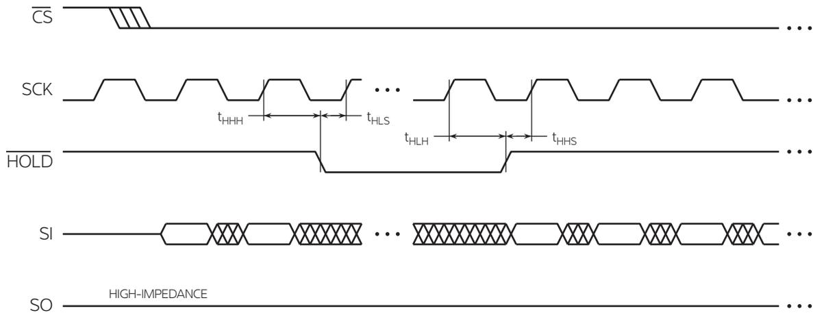
Figure 14-5.  $\overline{\text{HOLD}}$  timing – serial output
