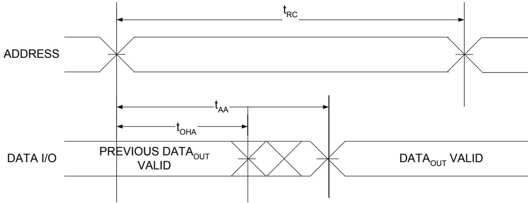
Figure 6. Read Cycle No. 2 ( $\overline{OE}$  Controlled)<sup>[14, 15]</sup>
