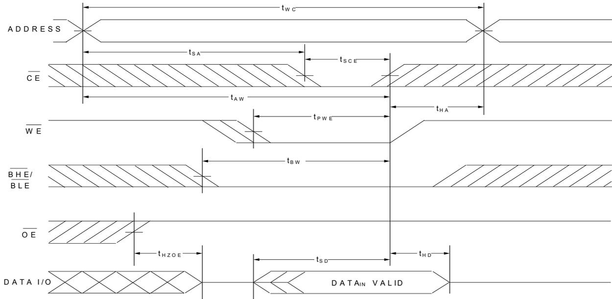
Figure 8. Write Cycle No. 2 ( $\overline{WE}$  Controlled,  $\overline{OE}$  LOW)<sup>[16, 17, 18]</sup>
