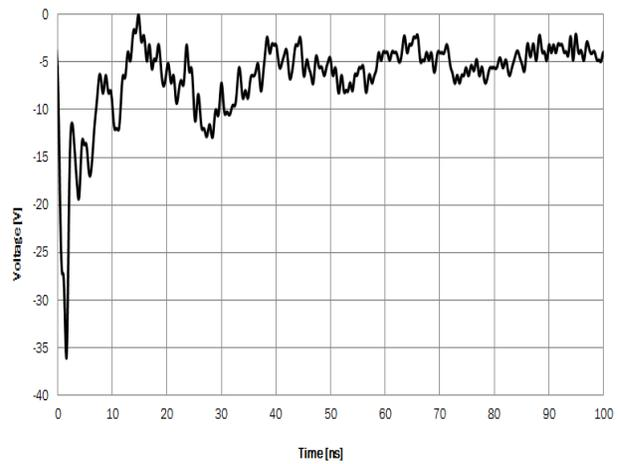
Figure 12. ESD5111 Negative 8 kV ESD Contact Discharge
