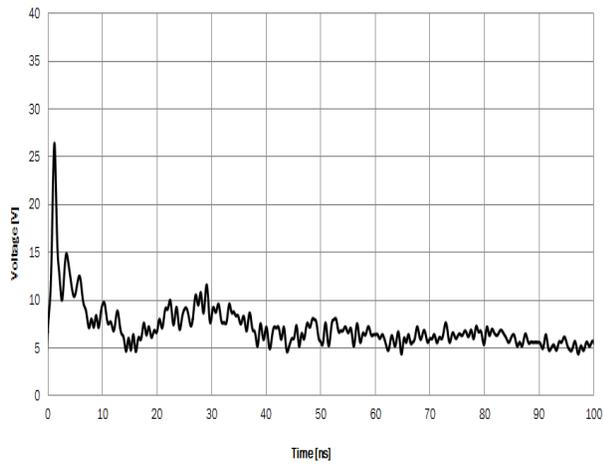
Figure 11. ESD5111 Positive 8 kV ESD Contact Discharge
