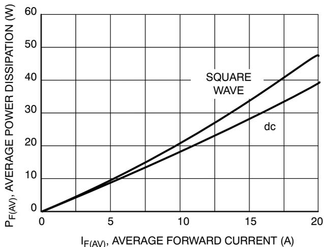
Figure 4. Power Dissipation
