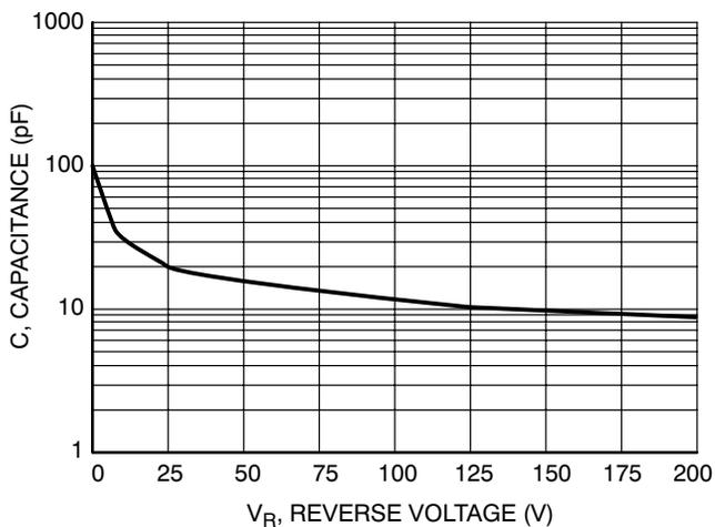
Figure 5. Typical Capacitance
