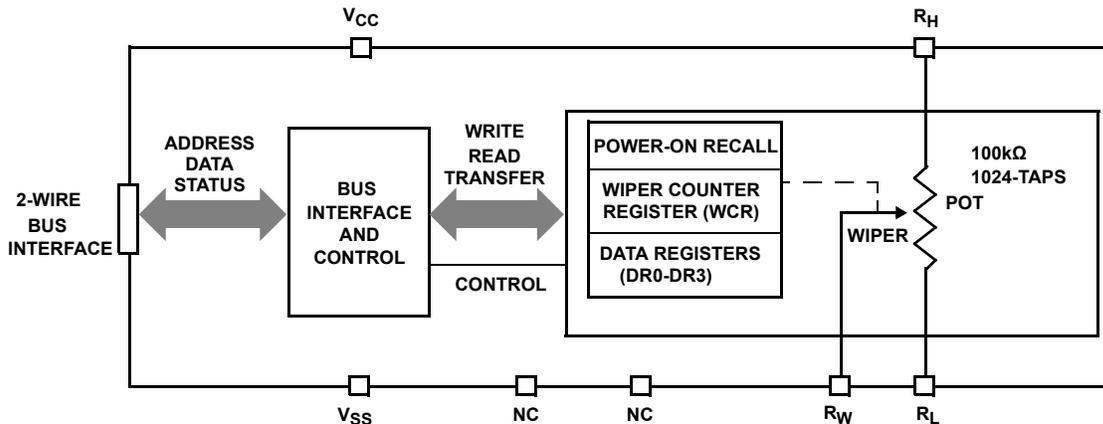
FIGURE 1. FUNCTIONAL DIAGRAM
