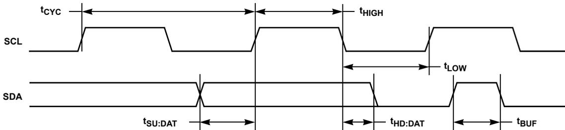
FIGURE 9. INPUT TIMING
