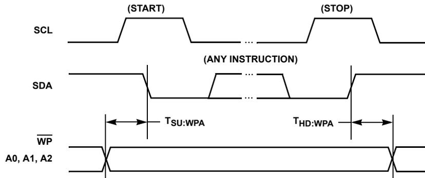
FIGURE 12. WRITE PROTECT AND DEVICE ADDRESS PINS TIMING
