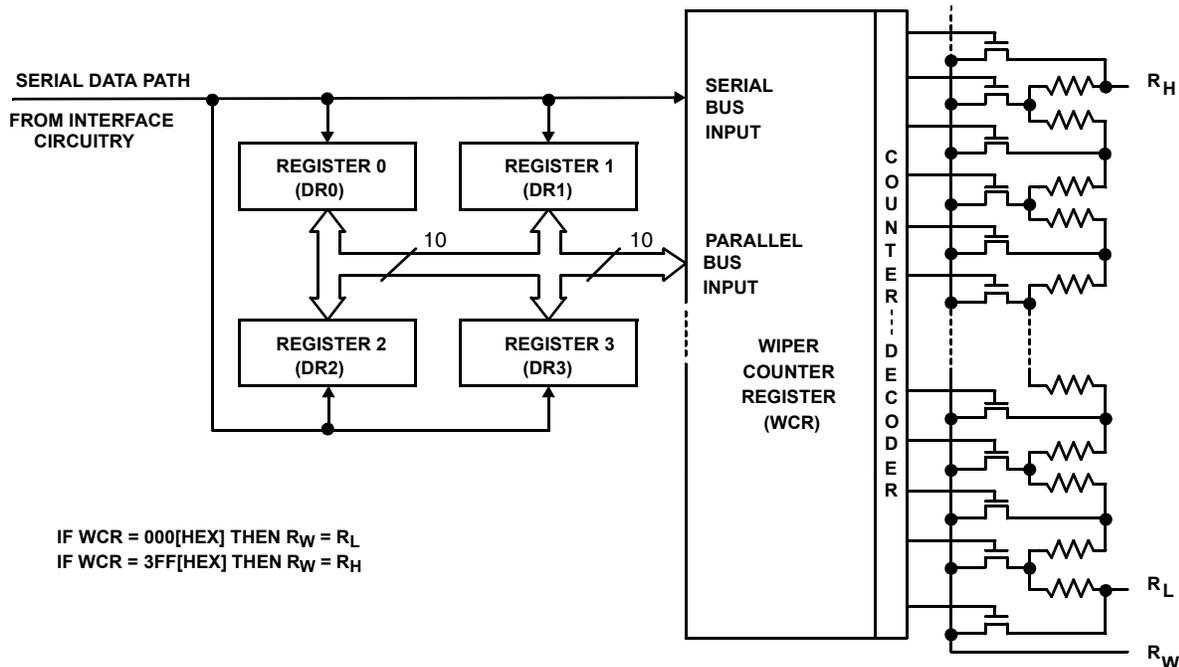
FIGURE 3. DETAILED POTENTIOMETER BLOCK DIAGRAM SERIAL INTERFACE DESCRIPTION
