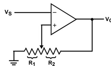
$$V_{UL} = \{R_1/(R_1 + R_2)\} V_O(\text{max})$$
