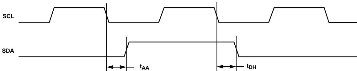
FIGURE 10. OUTPUT TIMING
