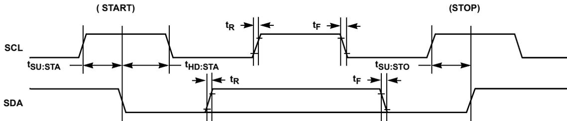
FIGURE 8. START AND STOP TIMING
