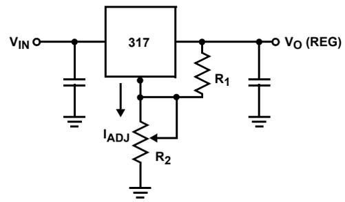
$$V_O (\text{REG}) = 1.25V (1 + R_2/R_1) + I_{\text{adj}} R_2$$
