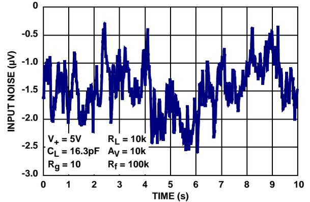
FIGURE 14. INPUT VOLTAGE NOISE 0.1Hz to 10Hz
