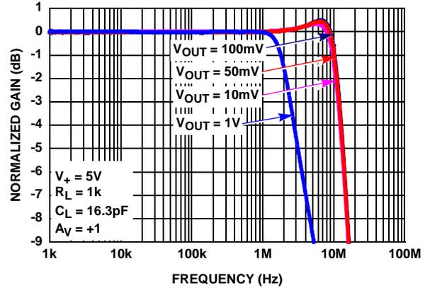
FIGURE 2. GAIN vs FREQUENCY vs  $V_{OUT}$ ,  $R_L = 1k$
