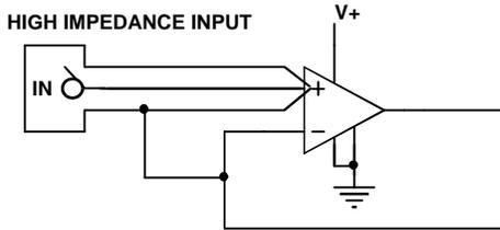
**FIGURE 44. GUARD RING EXAMPLE FOR UNITY GAIN AMPLIFIER**
