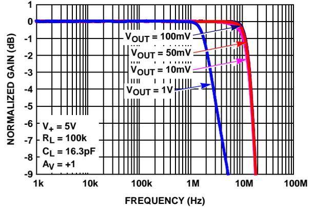
FIGURE 4. GAIN vs FREQUENCY vs  $V_{OUT}$ ,  $R_L = 100k$
