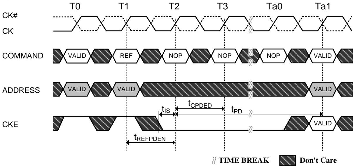
**Figure 62. Active Command to Power-Down Entry**
