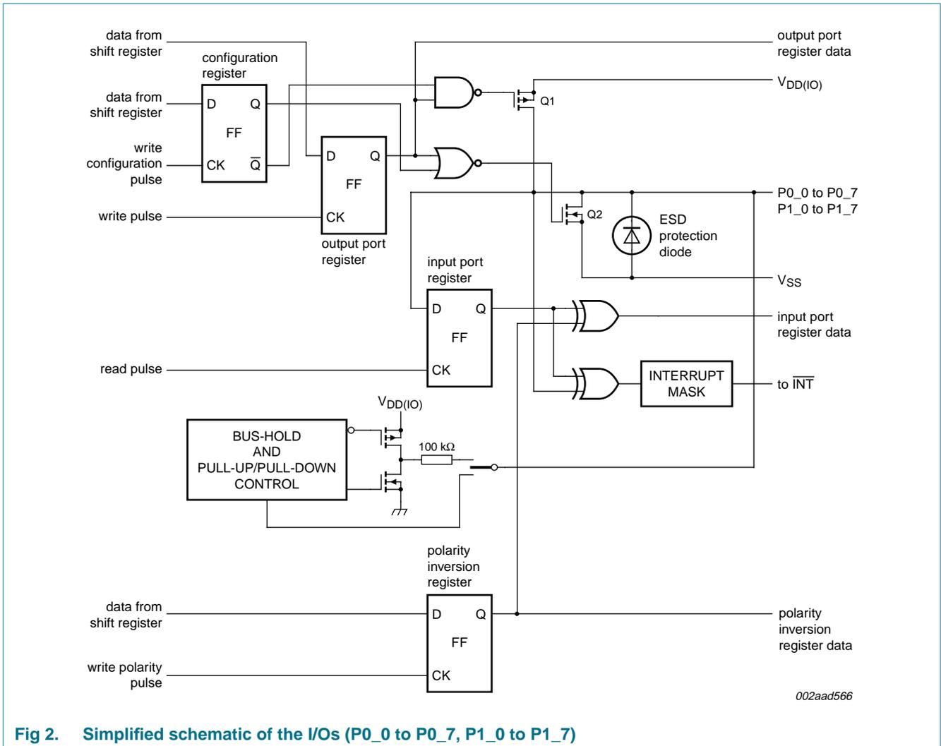
Fig 2. Simplified schematic of the I/Os (P0\_0 to P0\_7, P1\_0 to P1\_7)
