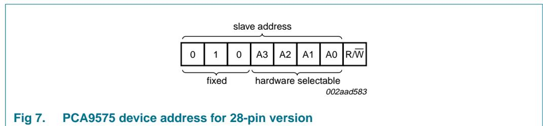
**Fig 7. PCA9575 device address for 28-pin version**
