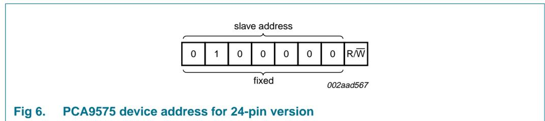
**Fig 6. PCA9575 device address for 24-pin version**
